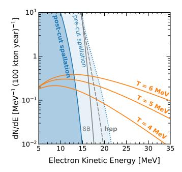
FIG. 8. DSNB  $v_e$  signal rates and background rates in DUNE, with nominal 7% energy resolution. Orange solid lines: DSNB signal rates, assuming neutrino temperatures of 4, 5, and 6 MeV. Light blue shaded: precut spallation spectrum. Dark blue shaded: postcut spallation spectrum (same as Fig. 5). Gray solid line: predicted <sup>8</sup>B event rates [1]. Gray dashed line: predicted *hep* event rates [1].
