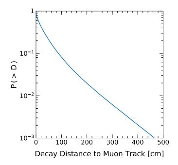
FIG. 4. Reverse cumulative distribution of spallation  $\beta$ s that survive from the first-step cut in perpendicular distance to the muon track.
