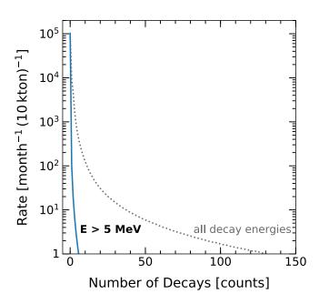
FIG. 13. Spallation isotope decay multiplicities per muon in DUNE. Bin size is 1 count. Gray dotted line: all spallation betas. Blue solid line: spallation decays above the 5-MeV threshold (in electron energy).
