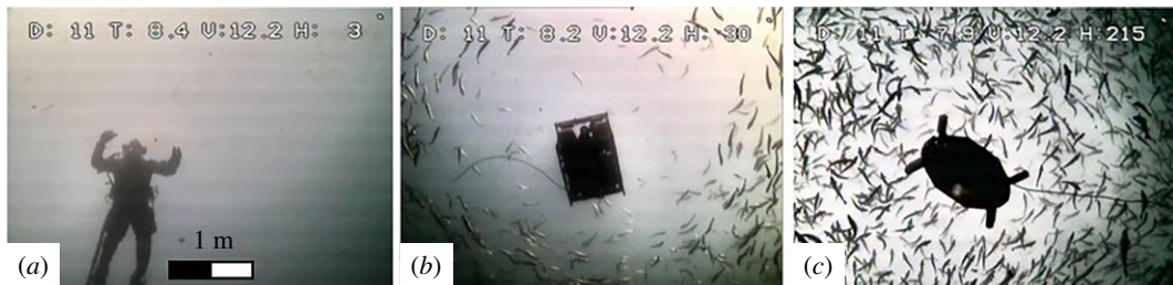
Figure 5. Frames from stationary camera filming the diver (a), Argus Mini (b) and U-CAT (c).
