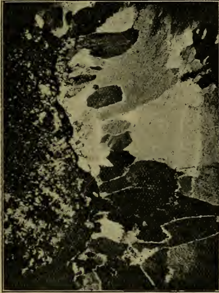
Fig. 3.— Metasomatic quartz, forming a fine-grained mosaic, accompanied by quartz filling a cavity, with comb-structure: Treacastell Mine, Conway. (Transmitted light: \times 50 .)
