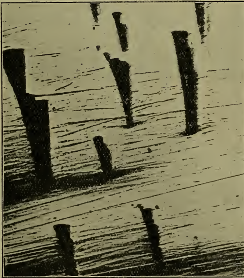
Fig. 6.— Etching figures on 'cubical' galena, oriented at right angles to the direction of polishing. (Reflected light: \times 200 .)
