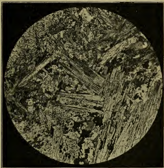
Fig. 8.—Section of a lenticle, magnified 23 diameters [14125], 1 showing mainly long sections of sillimanite.
