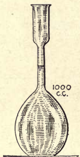
Fig. 2. — Liter Flask for Copper Assay.
