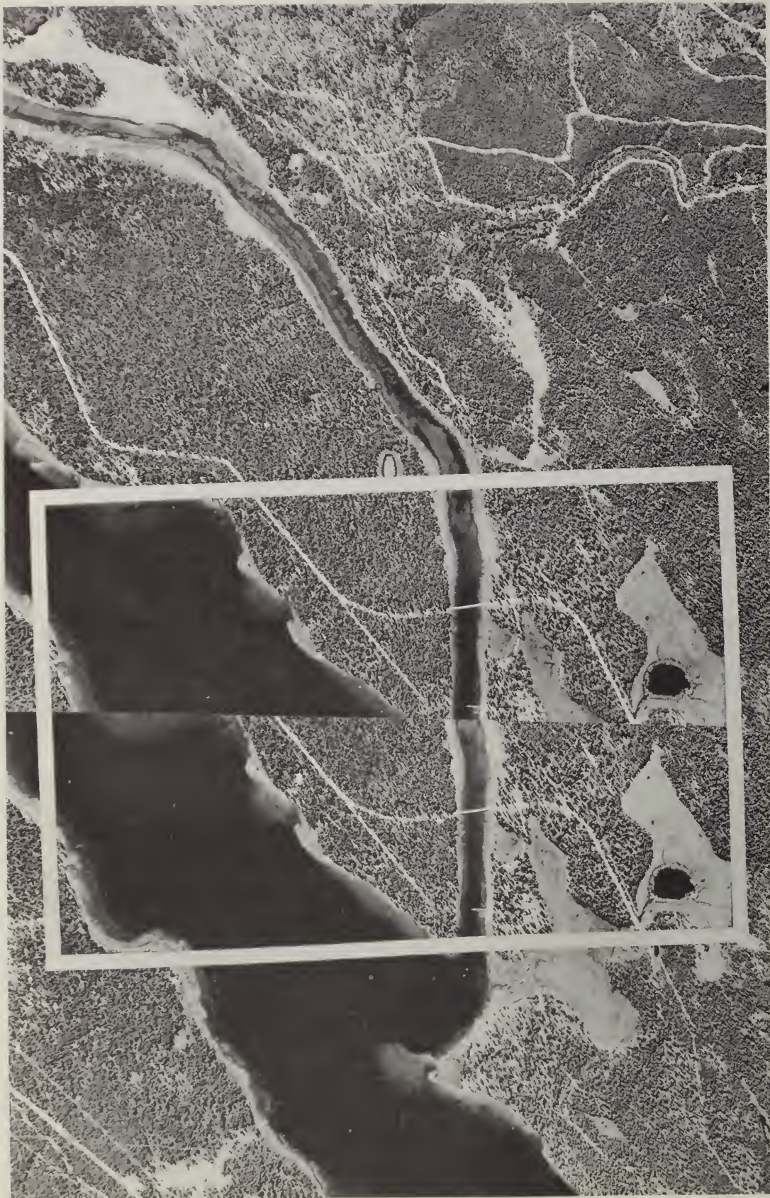
Figure 3.--Stereograms are prepared as shown. Photos are set up for parallax measurement. The area within the taped line is copied and used as a single print. Annotations may be entered either on the original photo or the copy negative.
