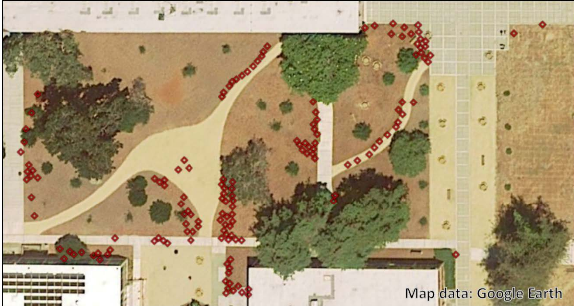
Figure 31. Locations of obstacles identified by the AGV. Adapted from [37].
