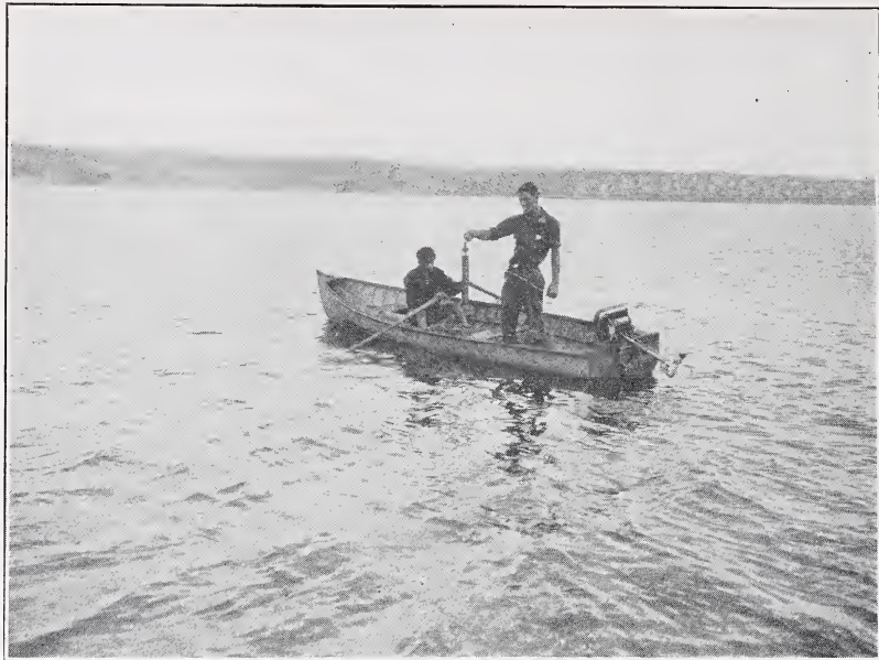
Lowering the water bottle to secure a sample of deep water for gaseous analysis
