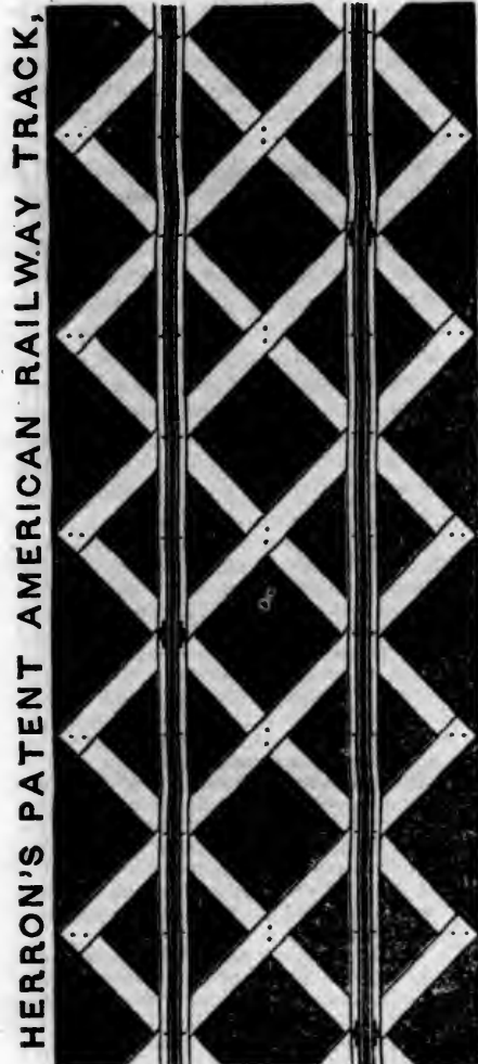
As seen stripped of the top ballasting.
