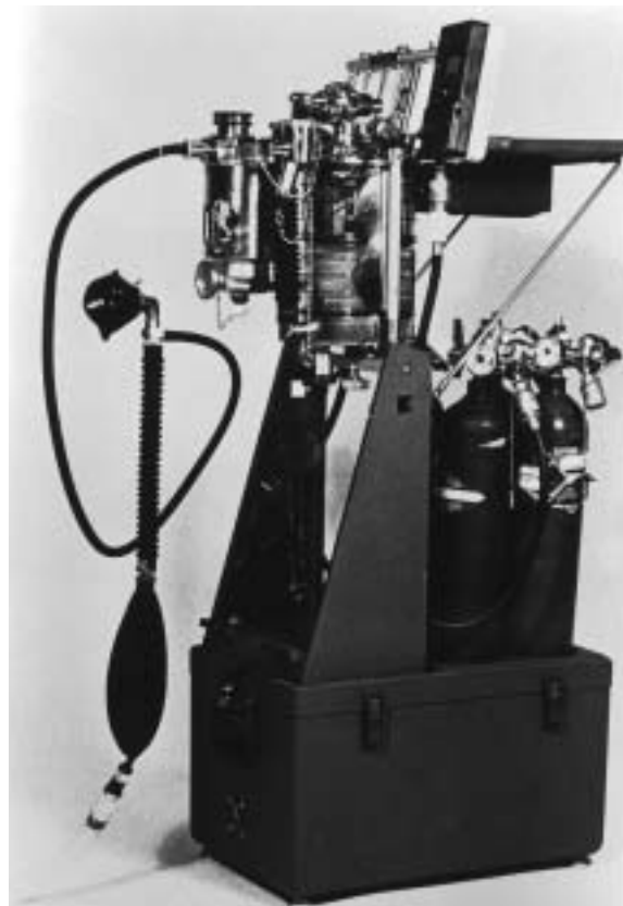
Fig. 7-38. Field Anesthesia Machine (FAM) Model 885A configured with a pediatric nonrebreathing circuit. Fresh gases flow from the outlet port near the vaporizer to the tee of the pediatric nonrebreathing circuit. The pop-off valve of the FAM is closed to prevent gas escaping to the atmosphere. Scavenged gases leave the tip of the rebreathing bag and flow into a corrugated hose. Photograph: Printed with permission from Ohmeda, Inc, Madison, Wis.
