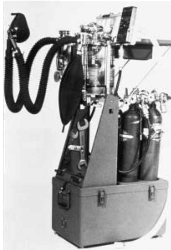
Fig. 7-2. Field Anesthesia Machine (FAM) Model 885A with an oxygen analyzer. The circle-system machine has a vaporizer, carbon dioxide absorber, flowmeters, and an adult patient breathing circuit. Compressed medical gases are required. Photograph: Permission granted by Ohmeda, Inc, Madison, Wis.
