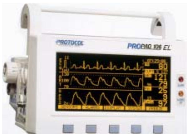
Fig. 7-60. PROPAC portable patient monitor. A unit this size can be fitted to monitor temperature, the electrical activity of the heart, pulse oximetry, blood pressure (direct and indirect methods), end-tidal carbon dioxide, venous pressure, and pressure from a pulmonary catheter. Photograph: Printed with permission of Protocol Systems, Inc., Beaverton, Ore.
