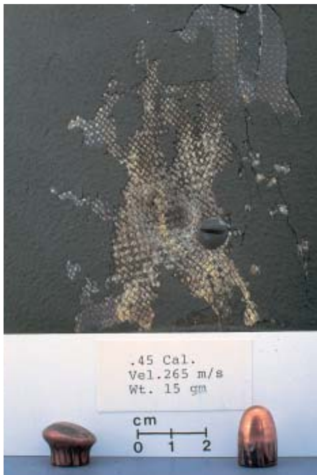
Fig. 16-1. The protection provided by Kevlar helmets is impressive: this helmet, seen close up, was struck by an 0.45 ACP (automatic Colt pistol) at a range of 3 m. The defeated bullet is shown on the left; an unfired bullet is shown on the right. By way of contrast, the 9 x 19-mm Parabellum round will usually perforate a Kevlar helmet. Photograph: Wound Ballistics Laboratory, Letterman Army Institute of Research, Presidio of San Francisco, Calif.
