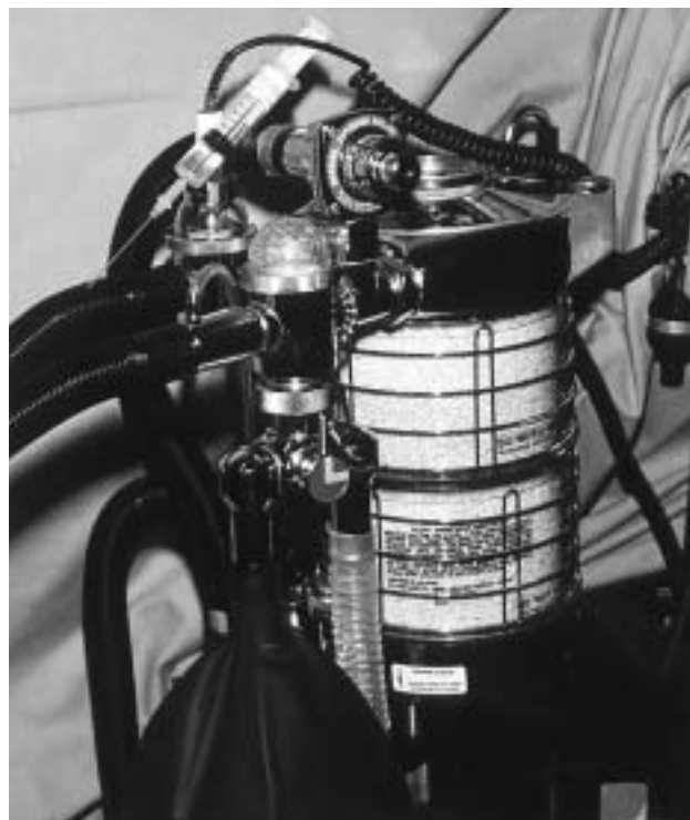
Fig. 8-8. Note the prominent label on this expedient liquid injector. The large needle facilitates filling the syringe and advertises that this is not a syringe intended for intravenous injection. The syringe remains in the circuit and is not placed with other syringes. If the syringe requires refilling, a new location in the tubing can be used for reinsertion.
