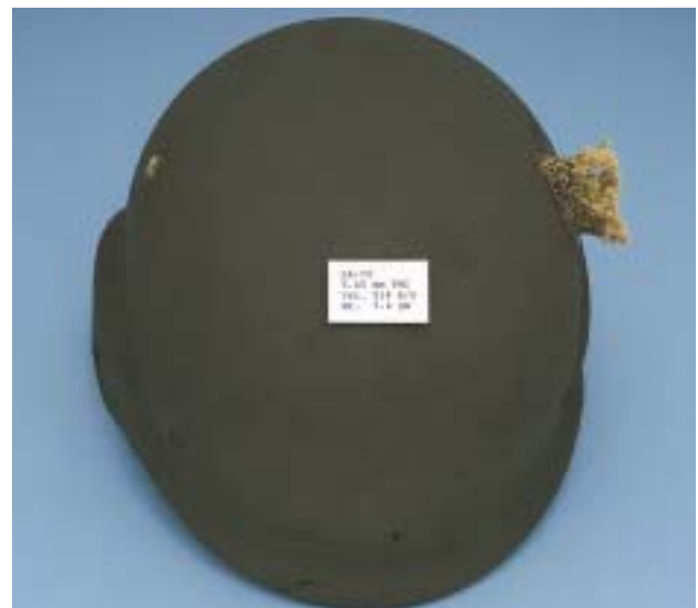
Fig. 16-2. Both sides of this Kevlar helmet have been perforated by a 5.45-mm bullet (fired by an AK74 at range of 3 m), which entered from the viewer's left. Notice the mushroomlike mass of disrupted Kevlar at the site of the bullet's exit. Kevlar fibers have been found lining tissue wound tracts in experimental ballistic studies. Photograph: Wound Ballistics Laboratory, Letterman Army Institute of Research, Presidio of San Francisco, Calif.
