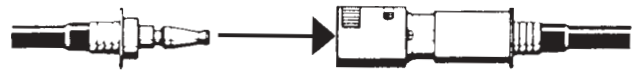
Fig. 7-23. Schrader noninterchangeable connectors at the ends of the gas hoses. Each medical gas has a specific connector assigned to avoid cross-connection of gases. One end of the gas hose has a male connector (left) that fits the gas-specific female connector (right) on the pin index safety system (PISS) regulator, and the other end has a female connector that fits the male inlet connection on the Field Anesthesia Machine (FAM) Model 885A. Schrader adapters allow rapid connections and disconnections without the use of special tools. Photograph: Printed with permission of Ohmeda, Inc, Madison, Wis.
