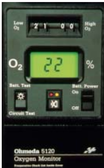
Fig. 7-49. An oxygen display of the percentage of oxygen in the gas mixture. Low-concentration and high-concentration alarms can be used by the anesthesia provider as conditions warrant. Photograph: Printed with permission of Ohmeda, Inc, Madison, Wis.
