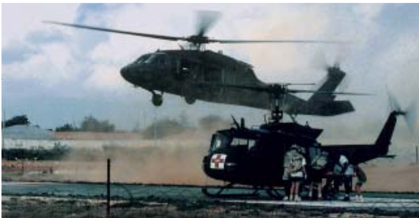
Fig. 27-5. A scene from the Somalia peacekeeping operation. A casualty is being removed from a UH-1 medical evacuation helicopter while a UH-60 hovers in the background. The latter is now the US Army's primary air ambulance, replacing the former, which has served with distinction since its introduction in 1959. The UH-60 has greater range and speed, and superior avionics compared with the UH-1 but, surprisingly, can carry no more casualties. Photograph: Public Affairs, Office of The Surgeon General, US Army.
