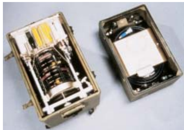
Fig. 7-7. Field Anesthesia Machine (FAM) Model 885A carrying case, opened. Bottom case (left) showing the FAM canister and rear of the flowmeter manifold. Upper case (right) with the medical gas hoses, a clipboard, and compressed gas regulators (one at each corner).
