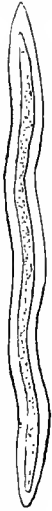
FIG. 116. — A wood fiber, consisting of a much elongated cell with thick woody walls.
