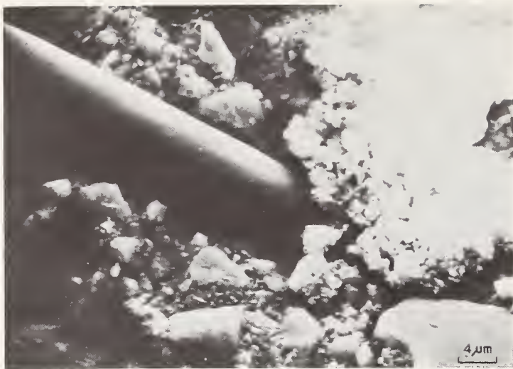
FIGURE 8. Scanning electron micrograph of a cement containing glass fibers. (National Physical Laboratory).
