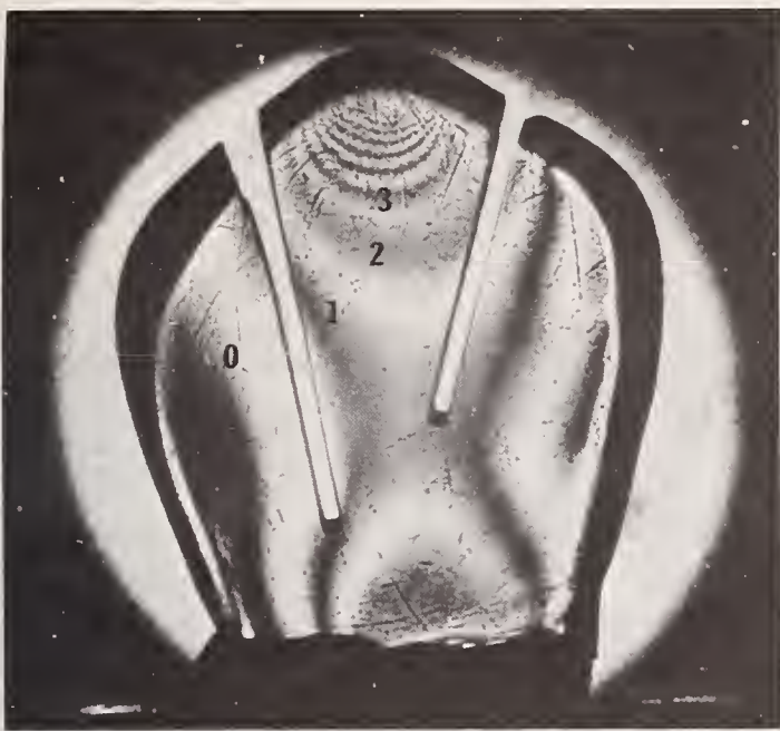
FIGURE 8. A slice from a three-dimensional model which has been subjected to a stress freezing cycle; isochromatic fringes are shown.
