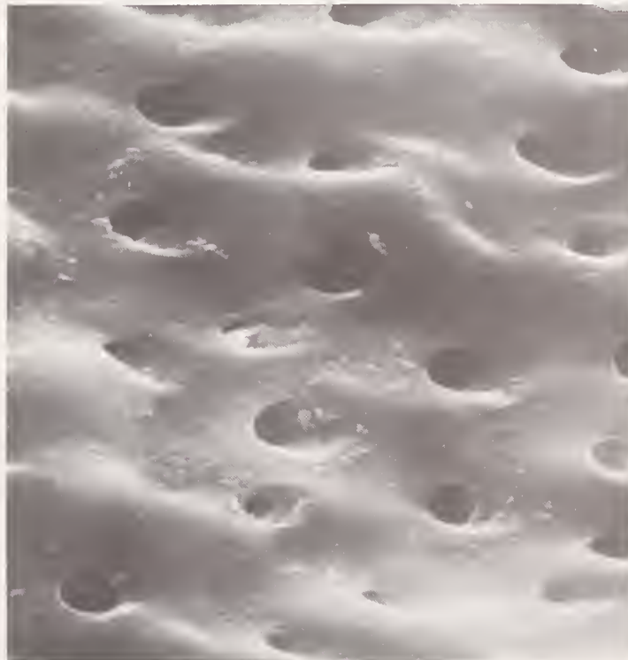
FIGURE 9. Bovine dentin treated with 50 percent aqueous formic acid for one minute (Magnification: 3000 \times ).
