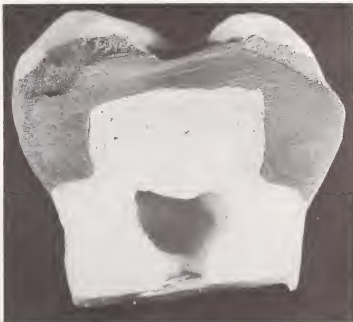
FIGURE 3. Section through an amalgam restoration condensed under 140 \text{kg}/\text{cm}^2 (13.8 \text{MN}/\text{m}^2 ) packing pressure against an \text{Al}_2\text{O}_3 reinforced EBA base with a ten-minute compressive strength of 470 \text{kg}/\text{cm}^2 (46.2 \text{MN}/\text{m}^2 ) [31].
