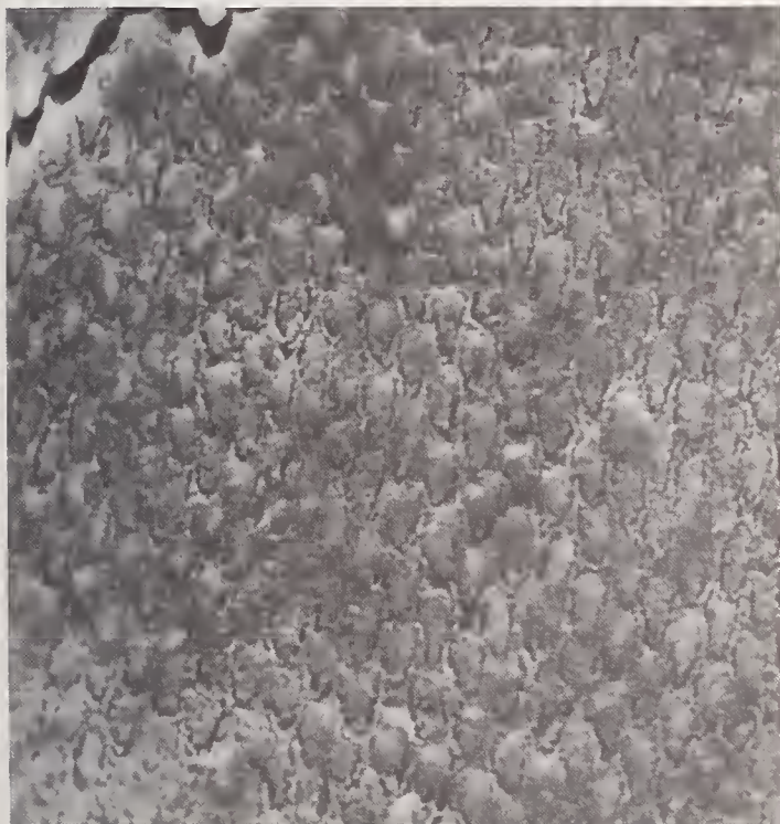
FIGURE 7. Bovine enamel etched with 50 percent aqueous formic acid for one minute (Magnification: 3000 \times ).
