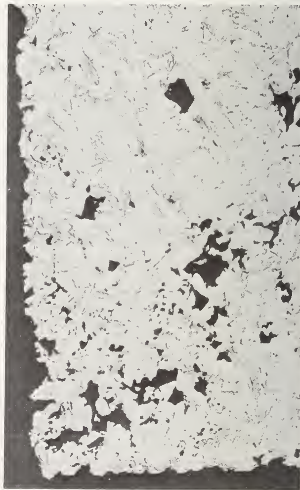
FIGURE 5. Porosity in the bottom corner of a well condensed, typical Class II filling made by a conventional technique. Magnification—approx. 115 \times .
