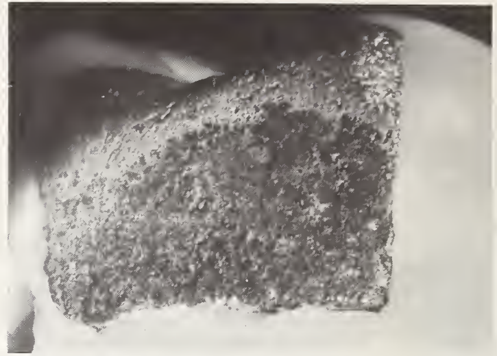
FIGURE 1. Typical corroded Class II filling with the gingival and central area covered by a crust of dark products of corrosion while the occlusal portion remains clear of corrosion.
