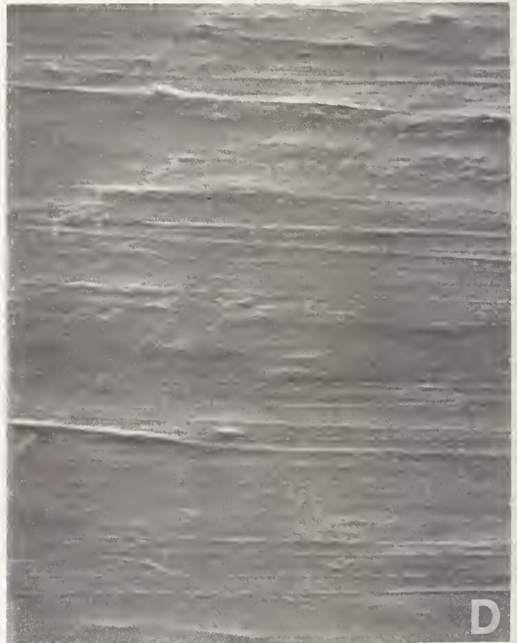
FIGURE 6. Bovine enamel polished with various abrasives (Magnification 9000 \times ). A: 220 grit paper ; B: 440 grit paper ; C: 600 grit paper ; D: \gamma -alumina.
