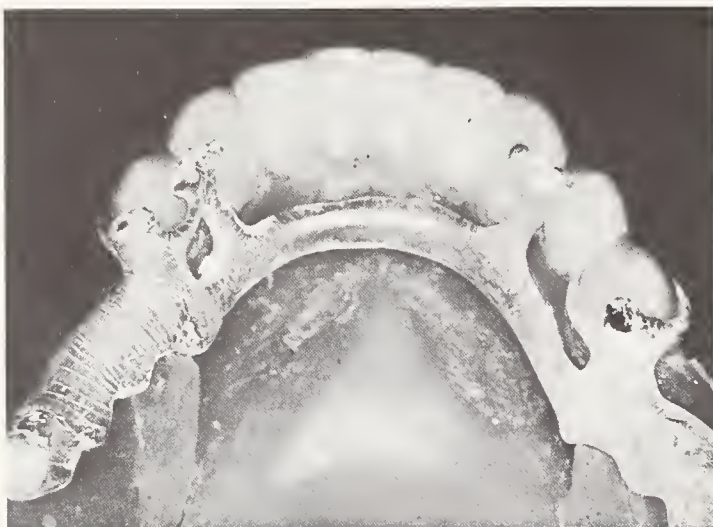
FIGURE 1. Mandibular partial denture framework coated with a brittle lacquer and loaded on the left posterior portion of the saddle.
