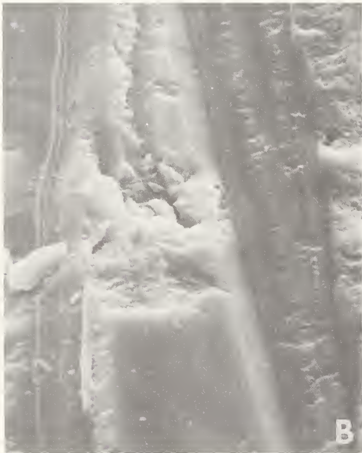
FIGURE 6. Bovine enamel polished with various abrasives (Magnification 9000 \times ). A: 220 grit paper ; B: 440 grit paper ; C: 600 grit paper ; D: \gamma -alumina.
