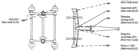
DOTTED LINE INDICATES LUBRICATION POINT ON BOTH SIDES.
