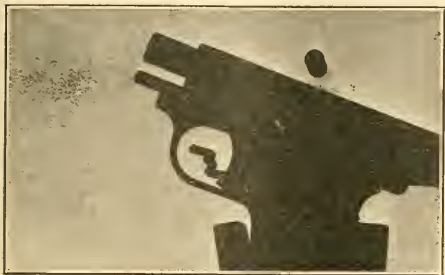
FIG. 3.—Automatic pistol; empty cartridge case ejected from receiver.
