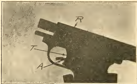
FIG. 1.—Automatic pistol in position of extreme recoil, empty cartridge case not yet ejected.
