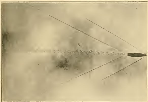
FIG. 4.—30 Calibre boat-tailed bullet, approximate speed 2500 feet per second.
