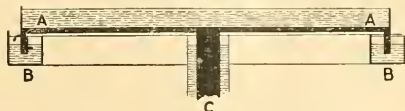
FIG. 3.—AA, Circular conducting plate and tank. BB, Annular hot water trough. C, Axis and cold-water tank.
