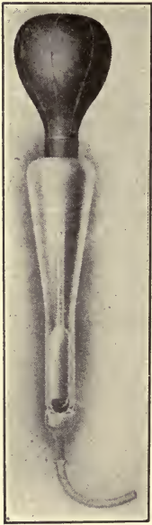
FIG. 172.—Hydrometer for testing the specific gravity of the electrolyte.
