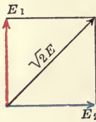
FIG. 255.—Voltage vector diagram for a two-phase alternator.
