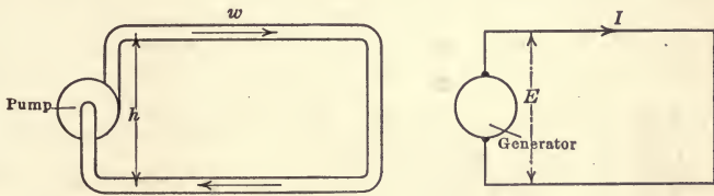
FIG. 21.—Hydraulic and electric circuits.
