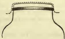
Fig. 164.— Top of Jar, with India-rubber band; place of tin cap shown by dotted line.
