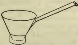
Fig. 166.—Funnel for filling Fruit Jars, with a rim set on below, to fit the outside of the neck.
