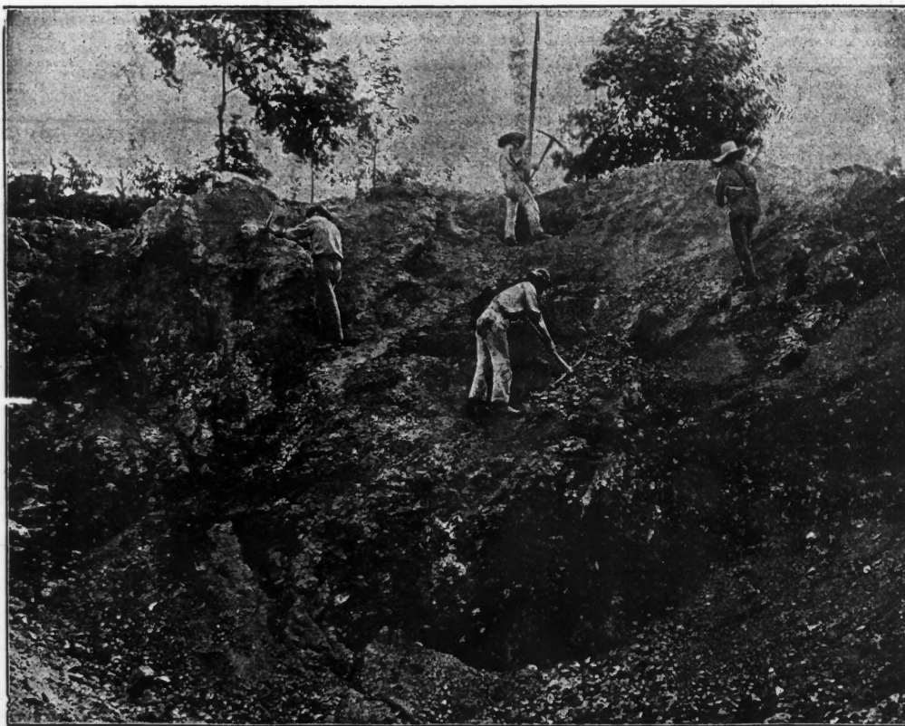
A hill of iron ore, the face of which has been uncovered to the depth of 40 feet. The base lies 200 to 400 feet below this.
