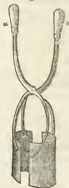
Fig. 2 shows a modification of the above instrument, wherein the blades are opened by moving the slider, *a*, upwards, and when thrust down around the plant, the blades collapse by pressing the slider downwards. The operation, afterwards, is the same as in Fig. 1.
