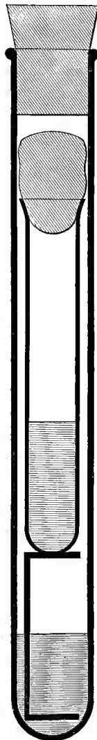
Buchner's anaerobic tube. The fluid consists of pyrogallic acid dissolved in 10 per cent. soda solution. By Wilson's method the tubes are charged with pieces of caustic potash covered with pyrogallic acid. (Park.)
