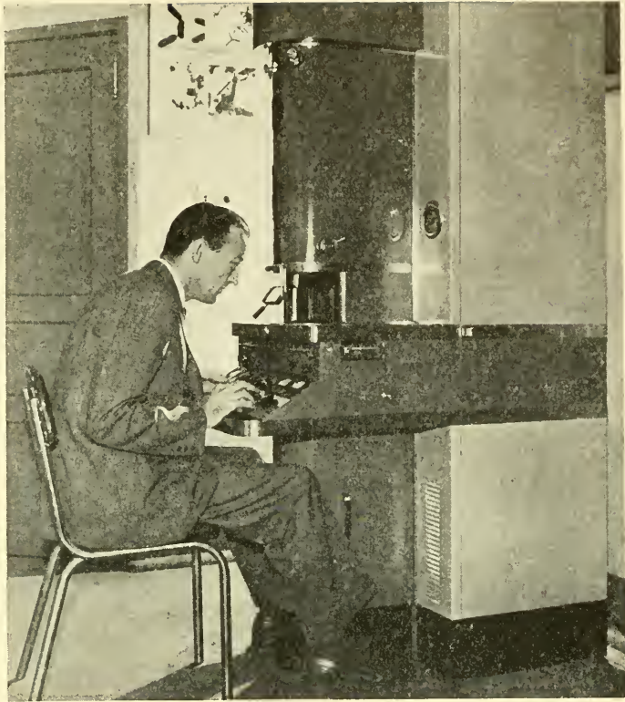
FIG. 10 The man is using an electron microscope. With its use it is possible to obtain photographs 200,000 times as large as the objects. You can see that the electron microscope bears no resemblance to the compound microscope. (R.C.A.)
