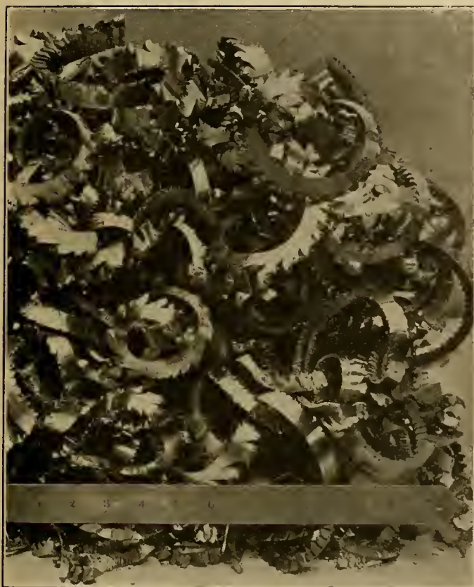
CHIPS FROM ROUGHING CUT ON A PAIR OF DRIVING WHEEL TIRES.
