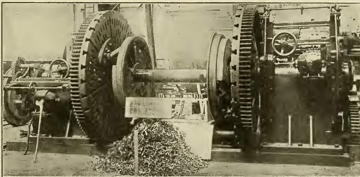
90-INCH NILES DRIVING WHEEL LATHE, OMAHA SHOPS—UNION PACIFIC RAILROAD.
