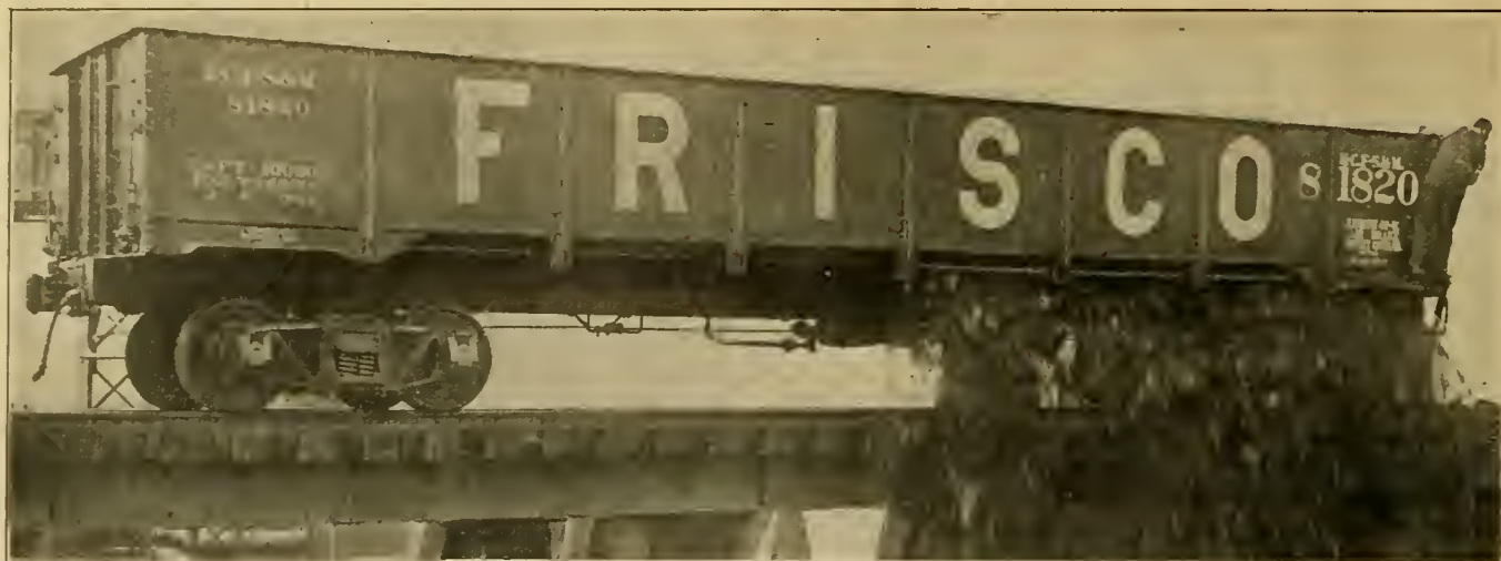
50-TON STEEL GENERAL SERVICE DROP BOTTOM GONDOLA CAR.
