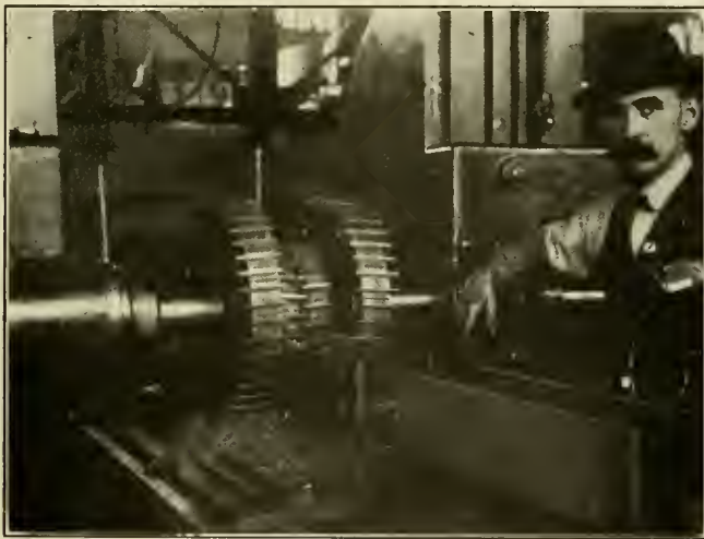
LARGE COMPOUND MILLING CUTTER FOR FINISHING SEVEN SURFACES AT ONE TIME.
