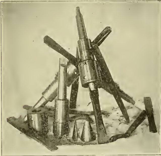
FIG. 14.—STANDARD CHUCK FOR HIGH SPEED FLAT DRILLS
