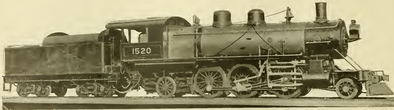
PRAIRIE TYPE LOCOMOTIVE, WITH WALSCHAERT VALVE GEAR—GREAT NORTHERN RAILWAY.
