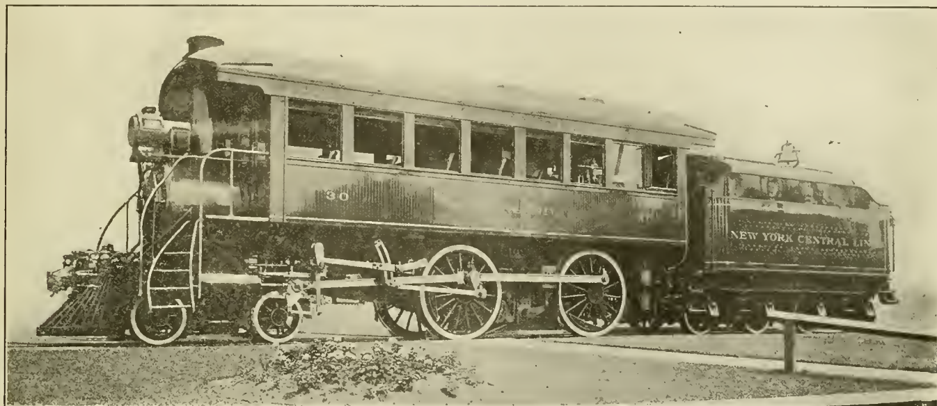
FOUR CYLINDER BALANCED SIMPLE INSPECTION LOCOMOTIVE, LAKE SHORE AND MICHIGAN SOUTHERN RAILWAY.
