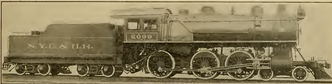
4-6-0 FREIGHT AND PASSENGER LOCOMOTIVE—NEW YORK CENTRAL & HUDSON RIVER RAILROAD.
