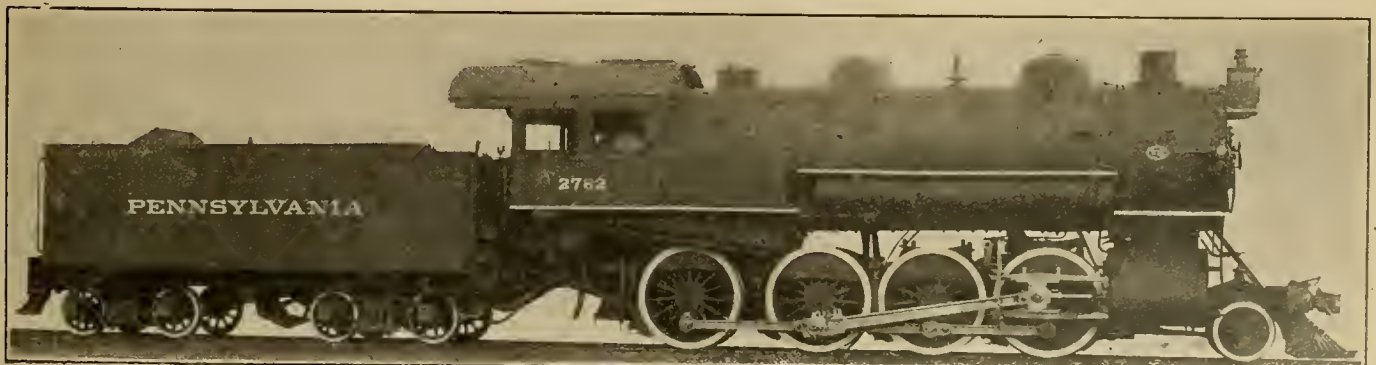
CONSOLIDATION (2-8-0 TYPE) FREIGHT LOCOMOTIVE—PENNSYLVANIA RAILROAD.
