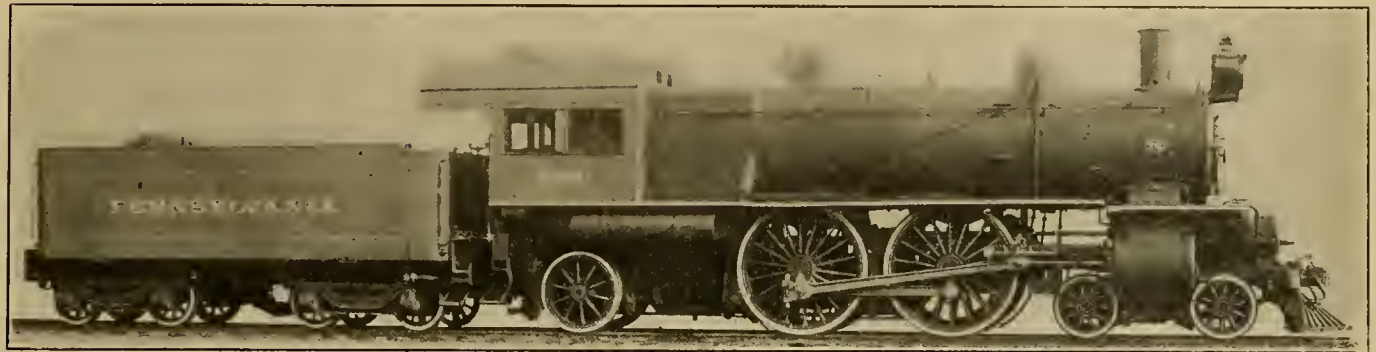
ATLANTIC (4-4-2) TYPE COLE BALANCED COMPOUND LOCOMOTIVE—PENNSYLVANIA RAILROAD.
