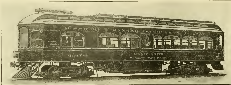
STRANG GASOLINE-ELECTRIC MOTOR CAR—SANTA FE TRAIL ROUTE.
