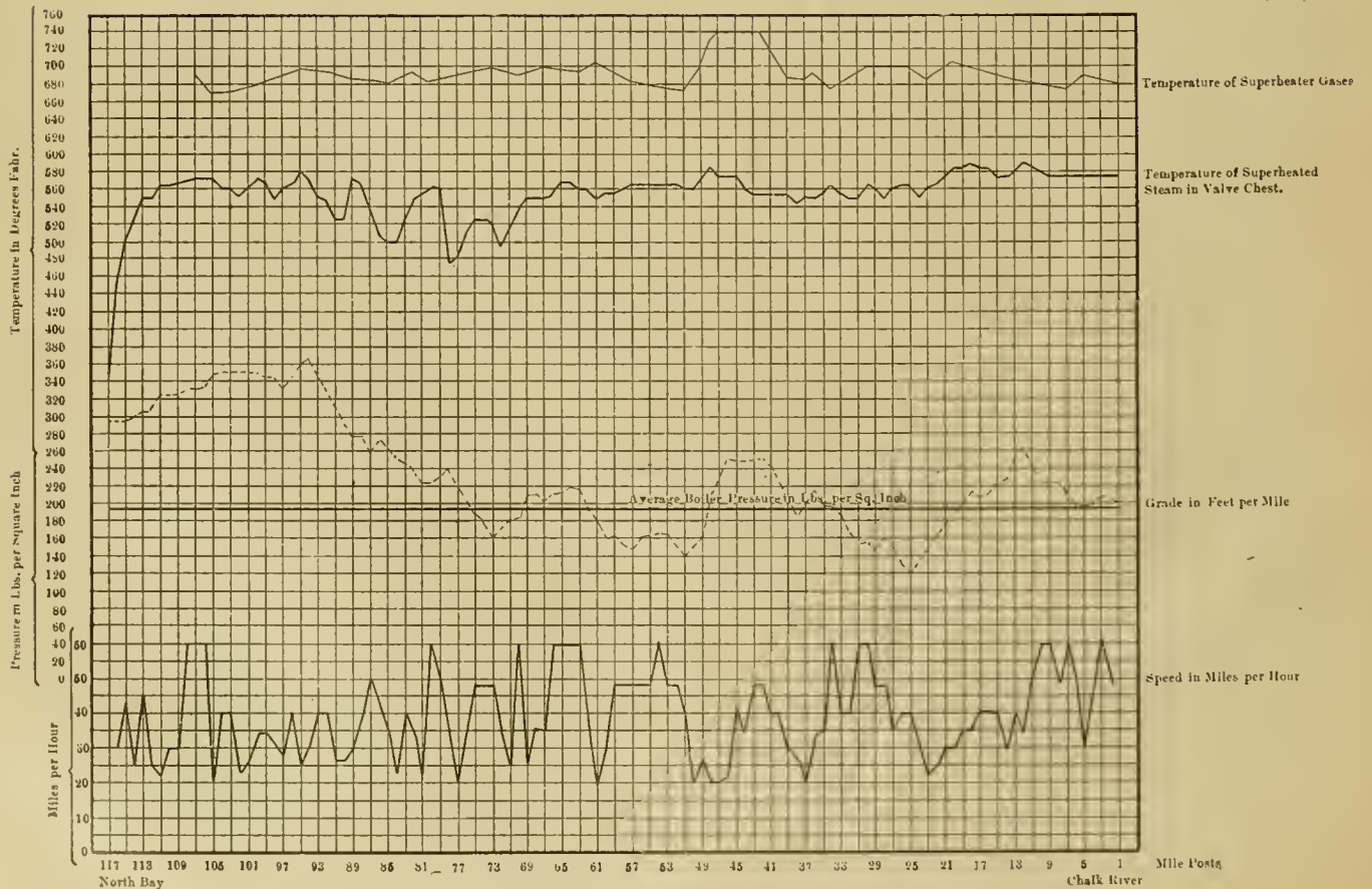
FIG. 3—TEST OF THE VAUGHAN-HORSEY SUPERHEATER—ENGINE 820, JUNE 27, 1905.
