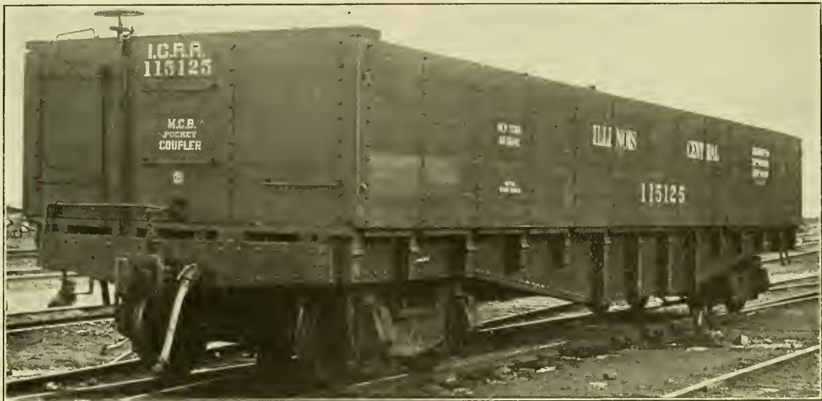
50-TON STEEL UNDERFRAME GONDOLA CAR—ILLINOIS CENTRAL RAILROAD.
