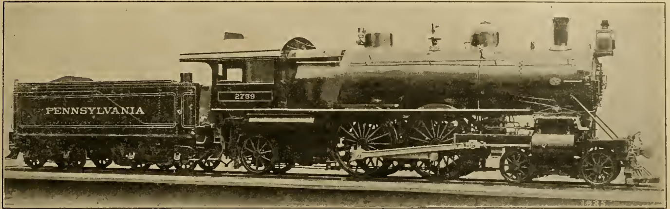
ATLANTIC (4-4-2) TYPE VAUCLAIN BALANCED COMPOUND LOCOMOTIVE—PENNSYLVANIA RAILROAD.
