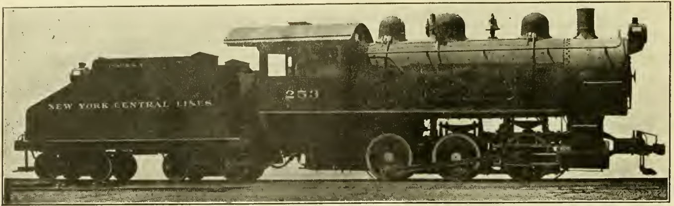
HEAVIEST 0-6-0 TYPE SWITCHING LOCOMOTIVE—PITTSBURGH & LAKE ERIE RAILROAD.
