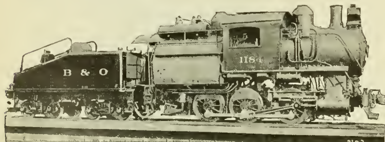
SIX-WHEEL SWITCHING LOCOMOTIVE.
