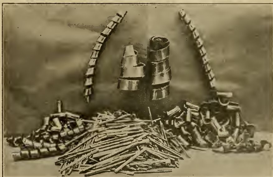
CHIPS FROM FINISHING CUTS. CENTER ONES AT REAR, 1\frac{1}{2} INCHES X 3-32 INCH; THOSE ON EITHER SIDE 1 INCH X \frac{1}{4} INCH; CENTRE ONES IN FRONT 3\frac{1}{2} INCHES WIDE FROM FORMING TOOLS.
