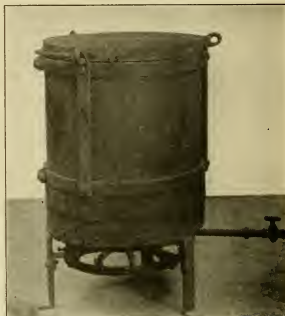
CIRCULAR FURNACE FOR HARDENING LARGE CUTTERS.
