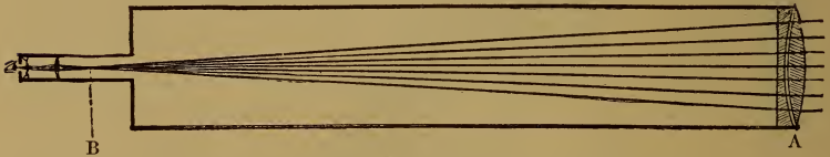
FIG. 86.—ILLUSTRATION OF THE PRINCIPLE OF REFRACTORS.
