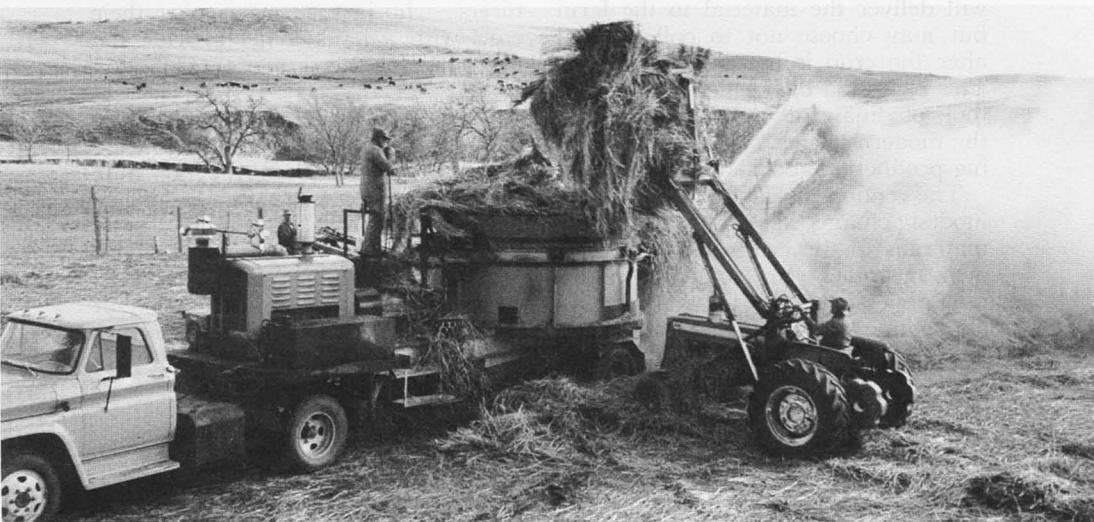
Custom operator stands on his hay grinding machine while rancher A. C. Smith on tractor feeds oats and barley hay into the "tub" grinder, in Corson County, S. Dak. Grinder's capacity is up to 15 tons of hay an hour.
