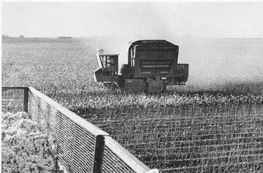
Cotton stripper-harvester of type used on Texas High Plains. A two-row stripper-harvester replaces about 100 men doing handpicking. Trailer load of cotton is in foreground.
