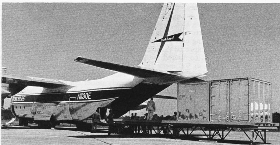
Small van containers being loaded through rear cargo hatch of prop-jet air freighter.
