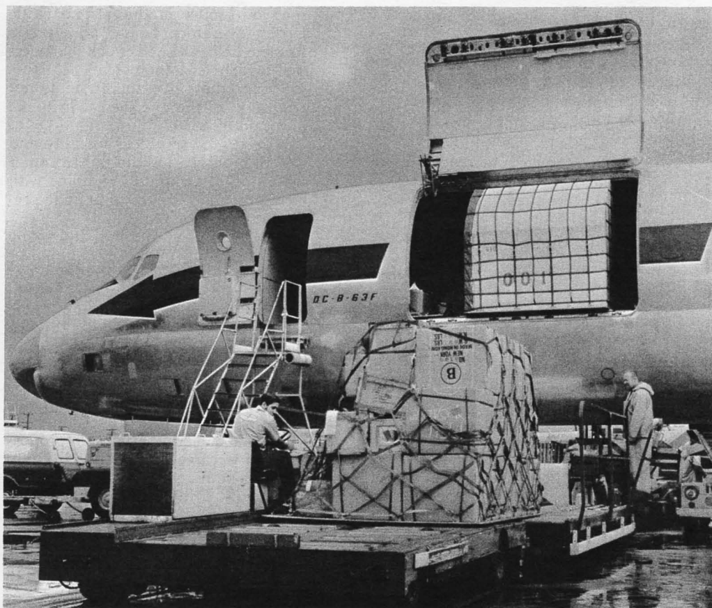
Fresh produce is either netted on pallets like cargo in foreground, or placed in "igloos" like one inside hatch of plane. Some growers prefer to lease their own igloos for direct loading at farm.
