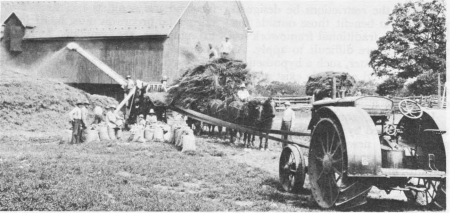
Thresher operating with power from tractor through a belt, probably in mid-1920's.
