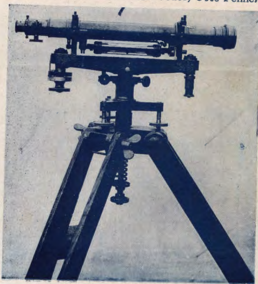
儀準水等二芬脫奧德 Levelling Instrument 2nd Order, Otto Fennel
