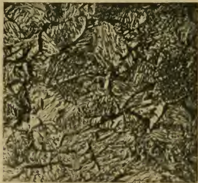
FIG. 2.—Hard-drawn gold wire after crystallisation at 280^{\circ} . Magnification \times 700 .
