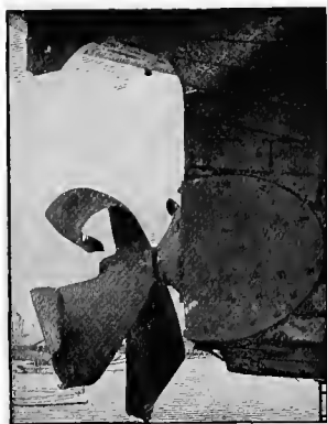
STERN OF THE U. S. S. NIPSIC Showing the Bent Propeller and the Loss of Rudder, Rudder-post and Heel
