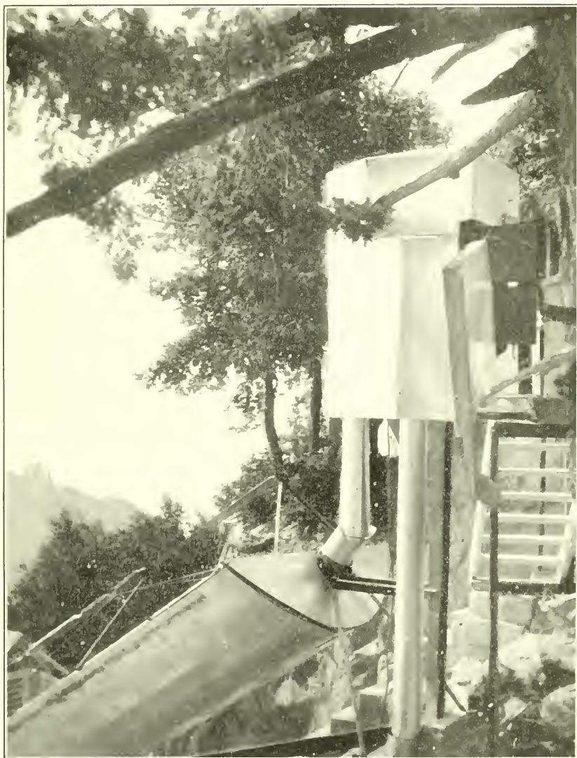
THE ABBOT SOLAR COOKER, MOUNT WILSON, CALIF. Side view showing end of great mirror, reservoir with ovens, and oil circulation tubes.
