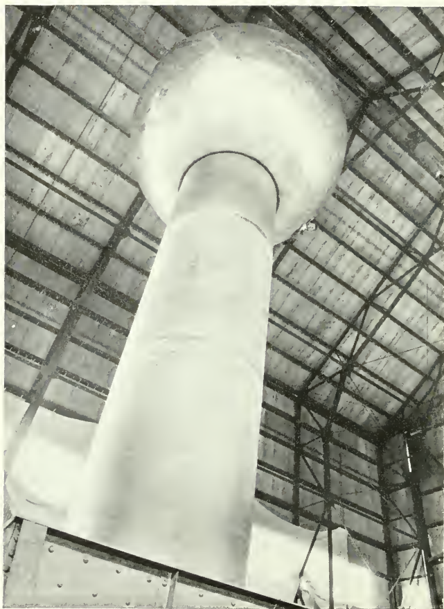
LOOKING UP ONE OF THE TWO GIANT SPHERICAL TERMINALS OF THE MASSACHUSETTS INSTITUTE OF TECHNOLOGY'S ELECTROSTATIC GENERATOR.
