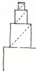
170. Failure of the method of similar dimensions, as applied to a storied tower.
