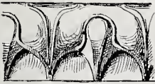
Fig. 23. Roman water-leaf moulding, from Pantheon: (probably from earlier Pantheon, 27 B. C., re-use in present structure.)
