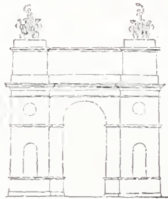
236. By an increase in relative size the piers count as the elements of a double group; the arch is reduced to a link between them. The arch should be still smaller than here shown, for due subordination.
