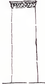
182. The proper cornice for such a front is the high one of slight projection.
