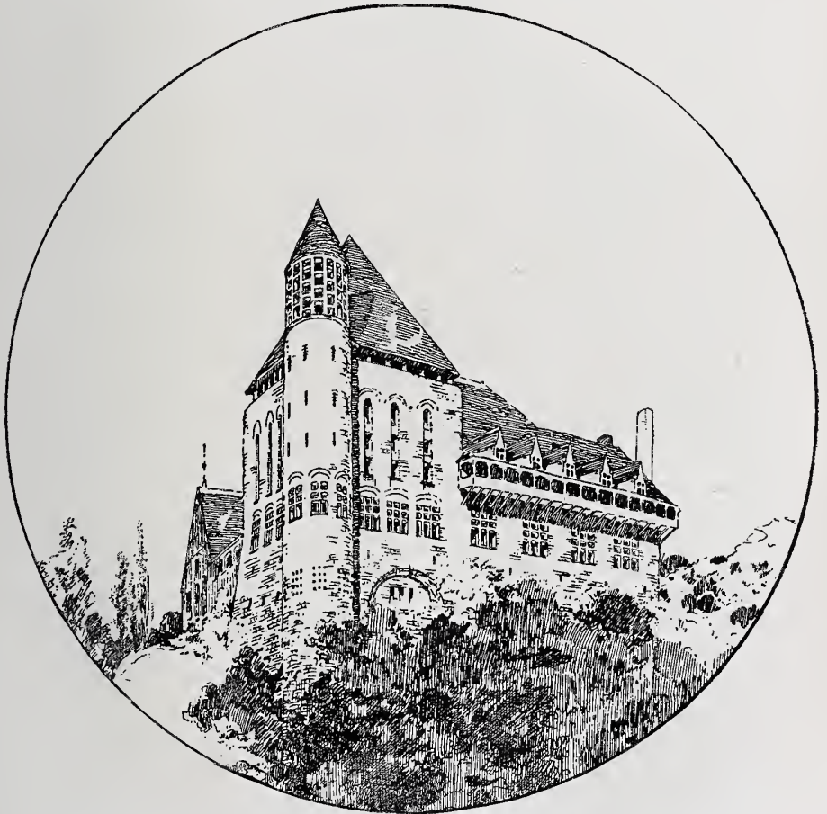
134. Design for Soldiers' Home, Minneapolis, Minn. L. S. Euffington, Architect. Grouping of windows. Triplet windows in mass. Four windows in appendage.
