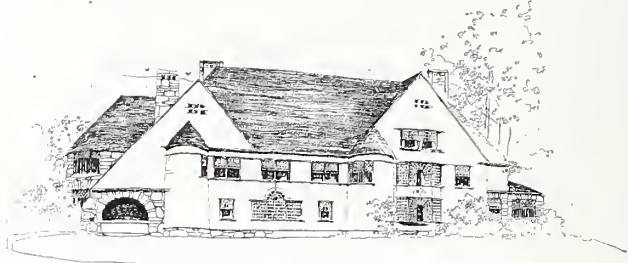
255. Double unsymmetrical group of gables, with an additional double symmetrical group of turrets.
