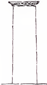
181. Bad effect of cornice of heavy projection on a tall and narrow front.
