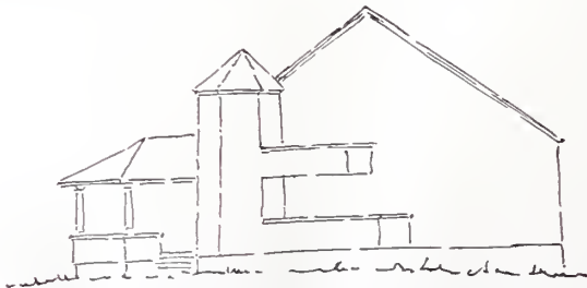
226. Elevation resulting from 226. The balconies are details, serving to connect the subordinate tower mass with the chief mass.
