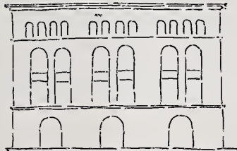
153. Variation of openings with continuous piers.
