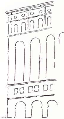
146. Large middle part formed by piers.
