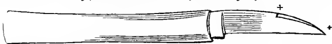
Fig. 195. Grafting-knife, with the portion of the back of the blade from + to + ground to a cutting edge, so as to make it serve also for a budding knife.
