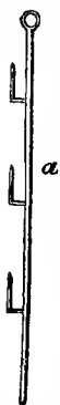
Fig. 266. Wire-standard for supporting rings, so as to form the frame-work shown in fig. 264.
