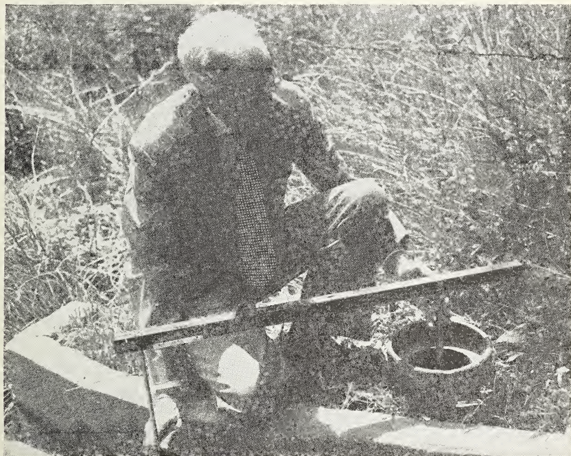
FIGURE 26.—The L-frame being used to check the datum point in stilling well. The rod at the left is resting on the midpoint of the crest; the \frac{1}{2} -inch square tube is resting on the washer datum point in the well. The level bubble at the center point of the horizontal leg of the frame is in exact adjustment. This datum point was originally set in May 1941. By loosening the wing nut at the left, the rod may be withdrawn and then inserted inside the \frac{1}{2} -inch square tube. These assembled parts are thereupon slipped into a deep groove on the underside of the horizontal leg of the frame and fastened in place by a slide-clip. This arrangement provides a convenient assembly for field use.
