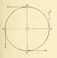
ond on an axis, o. If released at a, it flies off in the direction a b. The tendency to fly off is called *centrifugal force*. If the string be lengthened while the body is still revolving once a second, the force is increased. If the body be swung faster, the force is additionally increased. Hence, on a rotating sphere, centrifugal force is greatest at the Equator. If the rate of rotation be decreased, a body
