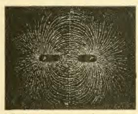
THE MAGNETIC SPECTRUM, SHOWING LINES OF FORCE.
