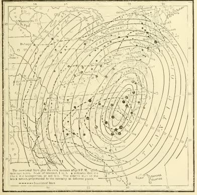
CO-SEISMAL AND ISO-SEISMAL LINES OF THE CHARLESTON EARTHQUAKE.
