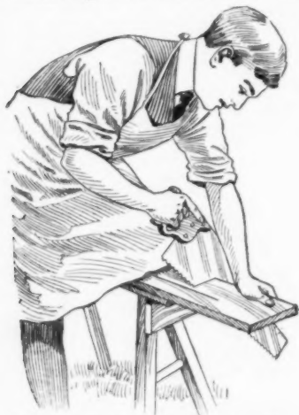
Fig. 17—Holding Overhanging Piece
