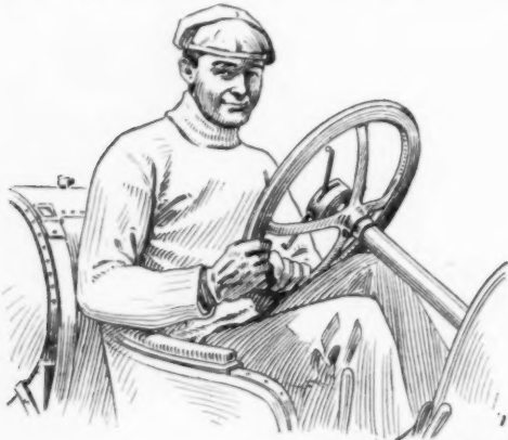
Courtesy the Automobile How Racing Drivers Hold Steering Wheel
