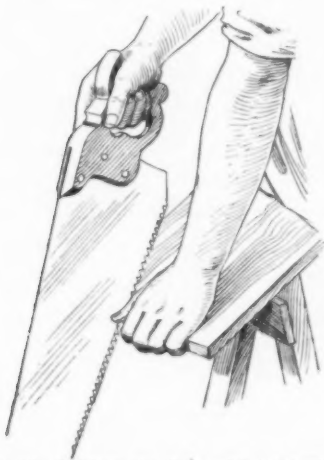
Fig. 14—Guiding the Saw with Left Thumb
