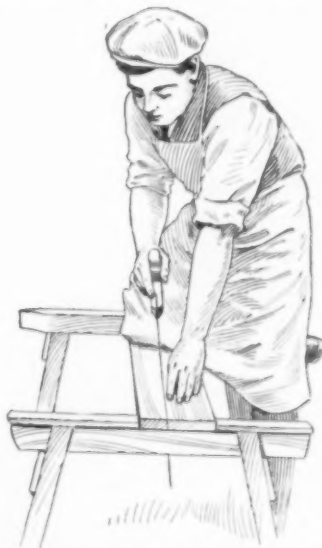
Fig. 16—Saw, Wrist and Elbow in One Plane
