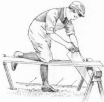
Fig. 15—Correct Angle of Saw
