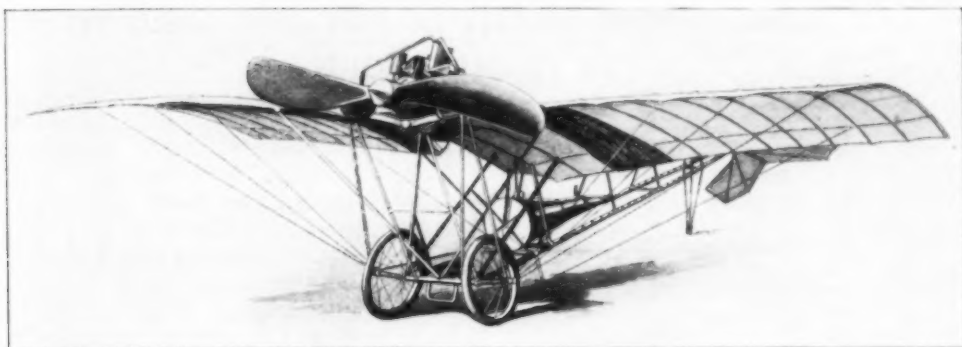
This View Gives a Good Idea of the Location of the Gasoline Tank and the Radiator
