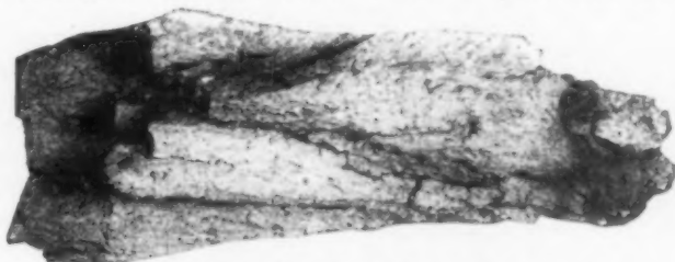
A Piece of Coke Made by the United States Geological Survey From Supposedly Non-Coking Coal
