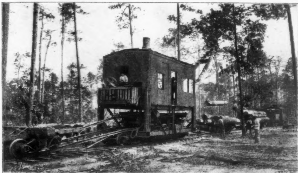
Hauls in Logs from Woods, Loads Cars and Makes Spur Tracks Unnecessary
