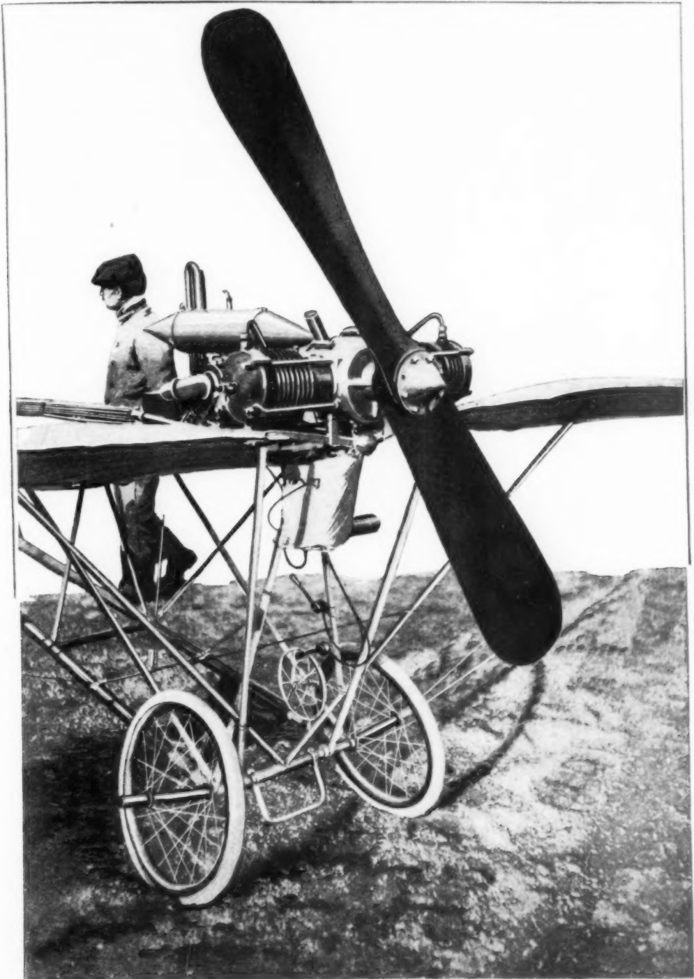
View of the "Demoiselle" Showing Position of Motor and Propeller
