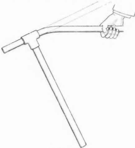
Bending a Pipe
