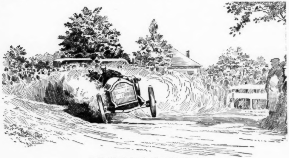
Inside Wheels Leaving Ground in Turning
