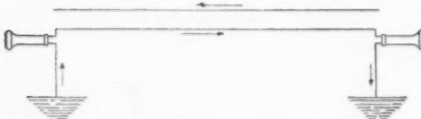
Fig. 3—Induction on Grounded Circuits
