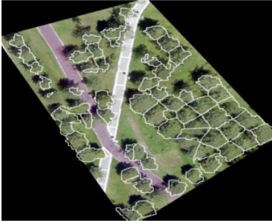
Figure 18. Illustration of result from performing RG segmentation. Source: Yilmaz et al. (2017).
