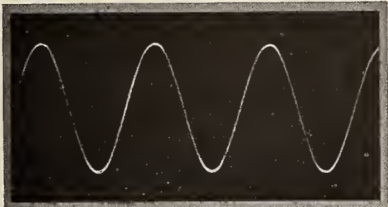
No. 1. Tuning Fork.—The tone of a scientifically mounted tuning fork is absolutely devoid of partial tones, hence the tone wave it creates is entirely free from the irregularities found in other tone waves, which are caused by their partial waves.
