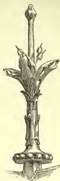
Épi of Lead, 13th century—Cathedral of Chartres. (From Viollet-le-Duc's "Dct. de l'Architecture.")
