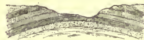
Section showing the erosion of the summit of a mass of stratified rock bent into a low anticlinal.
