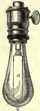
Incandescent Lamp, or Glow-lamp. a , carbon filament.
