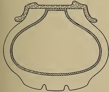
OVERLOADED 41%, NAMELY TO A TOTAL OF 1200 POUNDS, INFLATED WITH 60 POUNDS PER SQUARE INCH AIR PRESSURE
