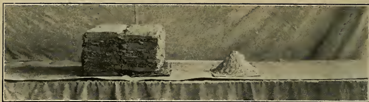
A WEIGHED-OUT RUBBER MIXTURE CONTAINING 100 PARTS RUBBER, 8 PARTS SULPHUR
