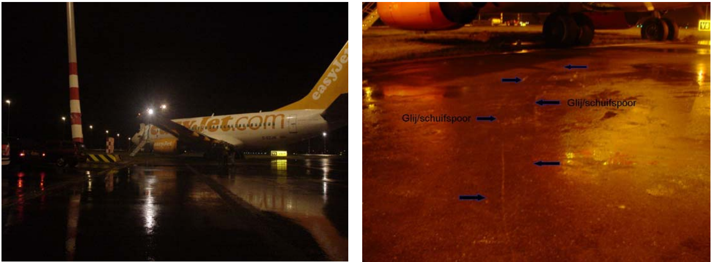
Figure 5: Photos of the aircraft after the accident and the tracks on the apron
