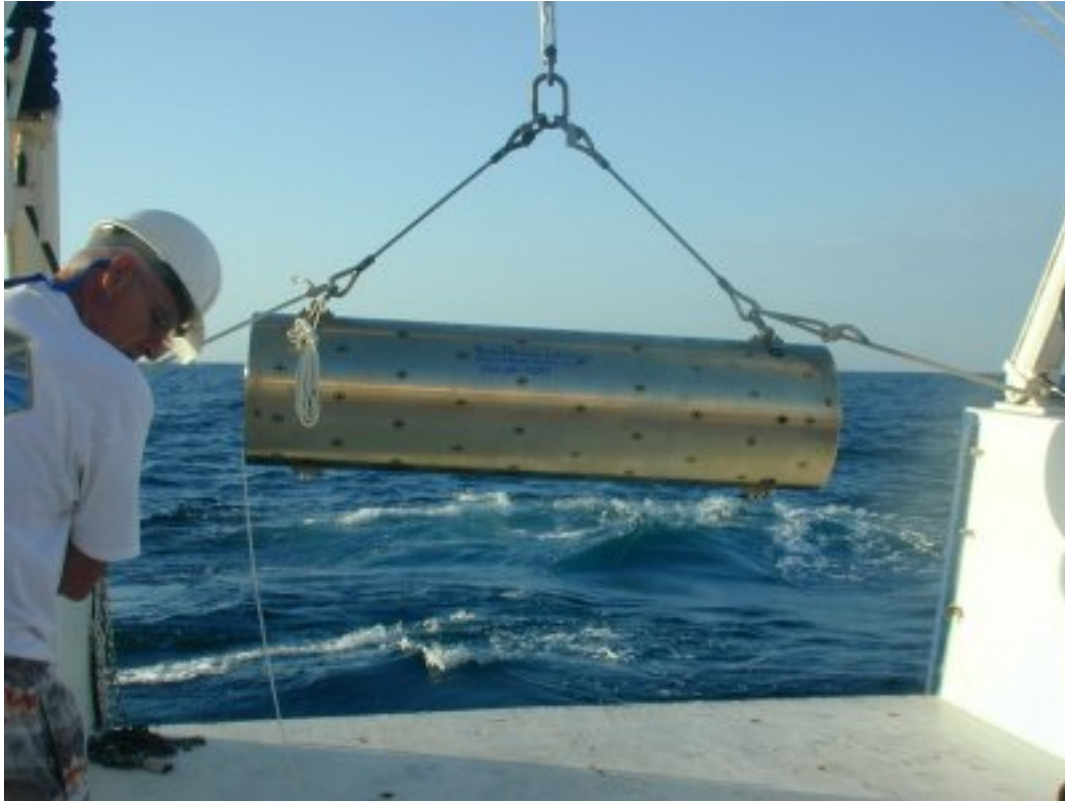
Figure 2.3 Acoustically Instrumented Mine (AIM) ready for deployment. Acoustic transducers, while visible, are seen to be flush with the hull of the mine (Photograph from OTI website, http://www.otiengineering.com/MineData/ ).
