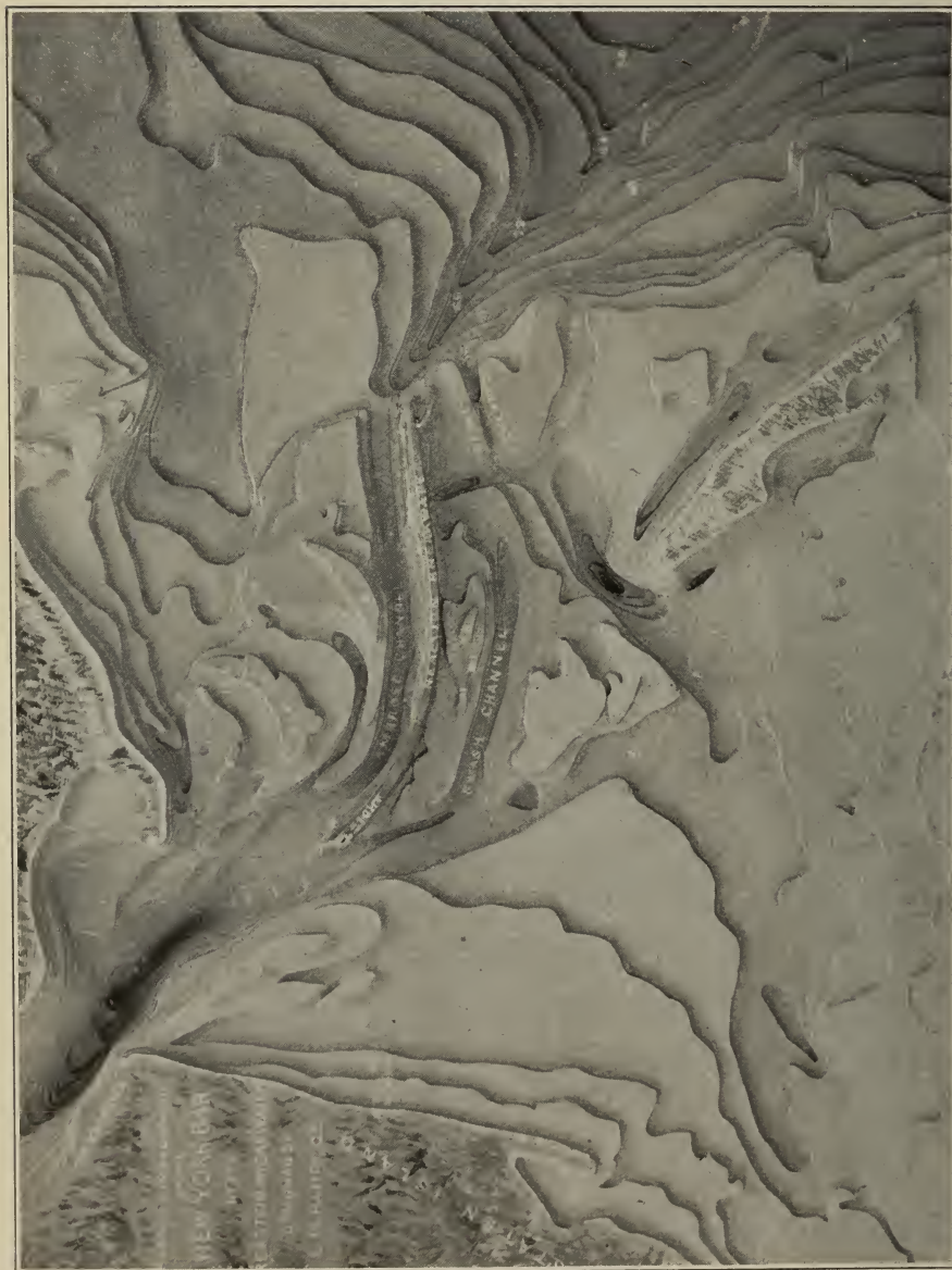
Model of Lower Bay, New York harbor, showing assumed effect on Ambrose channel of a proposed reaction jetty.—Six-foot contours.
