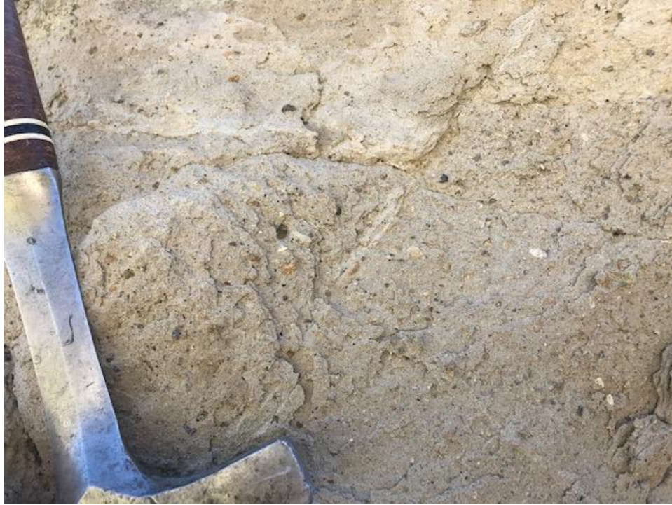
Figure 8. Close-Up of Silty Ash with Matrix-Supported Pebble-Sized Clasts, at Outcrop in Figure 7
