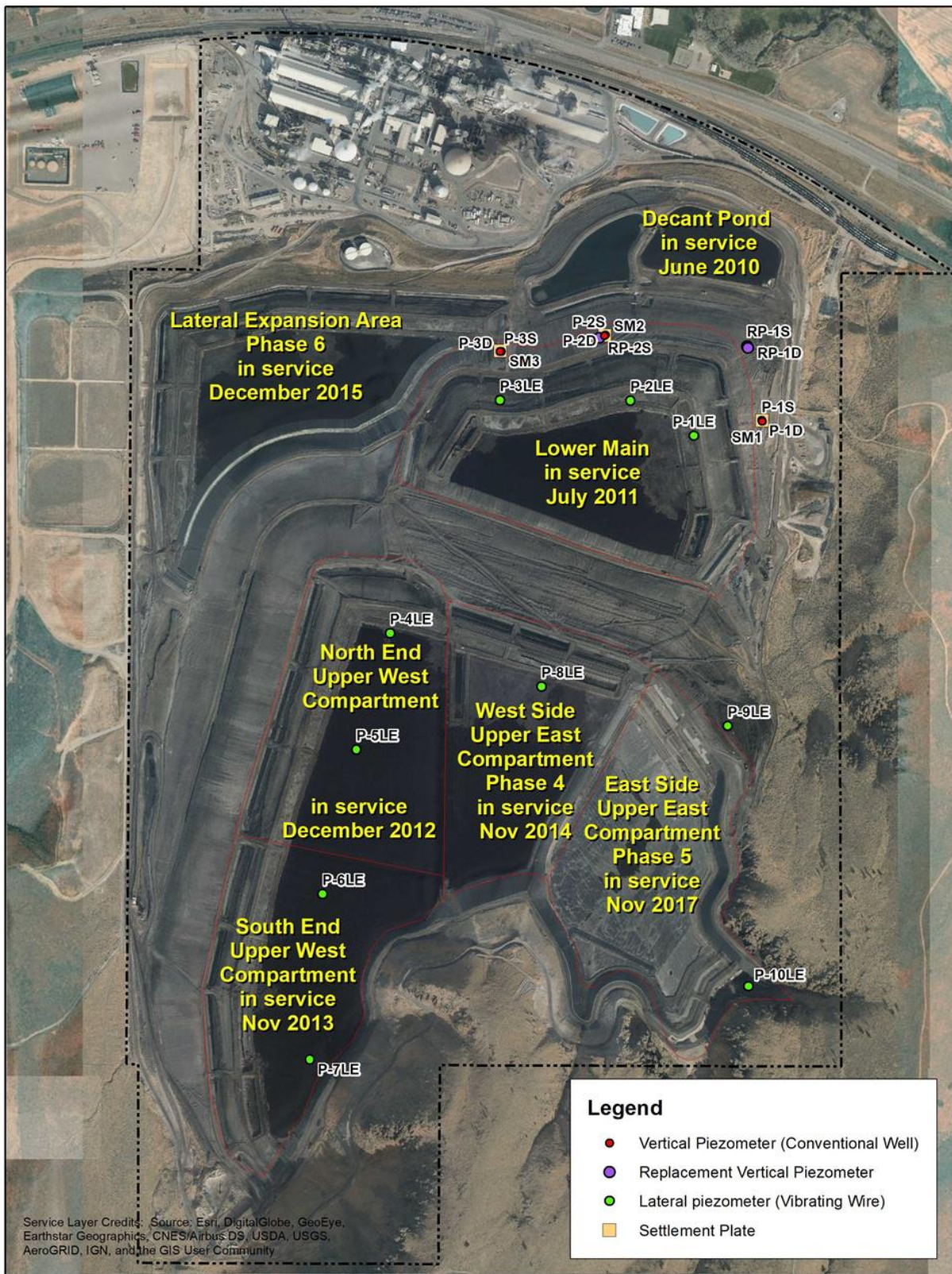
Figure 4-2. Gypsum Stack Layout
