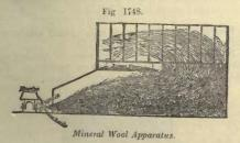
The slag is run into box cars, rolled to the wool-house, and there tapped. A small stream issues on to the runner, falls  $3_2^{1/\ell}$ , and is then encountered by a jet of steam which scatters it in threads into the house, which is  $30^{\ell} \times 40^{\ell}$ , and  $21^{\ell}$  to the comb. A sheet-iron extension  $10^{\ell}$  long reaches to the slag car. The size of the nozzle has an important bearing upon the formation of shot, as the pellets of slag are termed.
