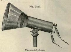
Ther'mo-phone. (Electricity.) An instrument in which sonorous vibrations are produced by the expansion of bodies under the influence of heat. One that produces sound by thermo-action through conversion of forces, or in other words, in rapid expansion and contraction of its circuit by sudden changes of temperature.
