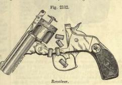
the hinge to uncover the breach, and throws the capsules clear of the barrels. The discharger then returns automatically into place
