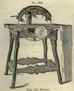
The inside of the saw fits into a groove on the driver which revolves the saw, so that the greater the amount of work on the saw, the tighter the friction holds it; and when the saw is not at work, the friction is only sufficient to revolve the saw. On the opposite end of the driving shaft from the friction wheel are two pulleys, tight and loose, to receive a 2½" driving belt. The saws can be used from ½" to 1" wide. See Fig 4334, p. 1945, "Mech. Dict." See also Rim Saw, supra.
