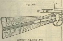
is heard, due to the head of the cartridge passing the cartridge stop. A sixth may be placed in the chamber. To load, turn the bolt and retract it. The bolt engages a cartridge, and the return motion forces the load into the chamber and cocks the piece. The piece has the usual 4 motions: Twist, draw, return, lock. The cocking being automatic, the piece is ready to fire.
