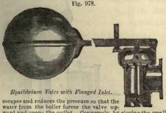
water from the boiler forces the valve up-ward and opens the outlet. Conversely, by closing the small valve the operation is reversed.
