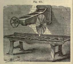
Bracket Cutting-off Saw, with Traversing Arbor.
