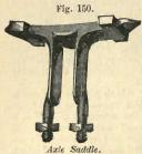
curing a spring to an axle. A plate or yoke slips over the screwed ends, and is secured by burs.
