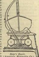
iron rafts which these ves-sels all carry. The rafts (American Steamship Co) are stowed under the boats, the whole being very compactly arranged, but always ready
