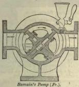
ing abutment H, which moves back and forth on its seat with the throw of the eccentric ring E. The tumblers fitted to this abutment adjust themselves to the ring, and as the pressure is constant upon them from above, they effectually pack the ring and prevent any escape of water below.
