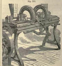
Holmes's Barrel-chamfering, Crozing, and Howeling Machine.
