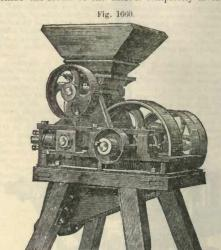
Malt Crushing Mill.
