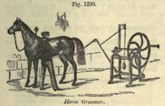
jointed revolving shaft to rotate a brush used in
