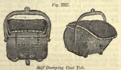
right position, but when the end of the track is reached the weight turns them on the tubs' axes and dumps them.
