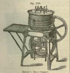
the pan. The knives are moved vertically by means of an axial rod passing down through the center of the chopping block and attached to a crank-pin beneath. The block has an intermittent motion in the interval between the cuts.
