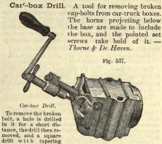
tance, the drill then removed, and a square drift with tapering edges substituted in the spindle and forced into the hole by the feed-screw, until its edges are slightly imbedded in the bolt. By turning the crank and feed-screw in the reverse direction, the broken bolt will be readily backed
