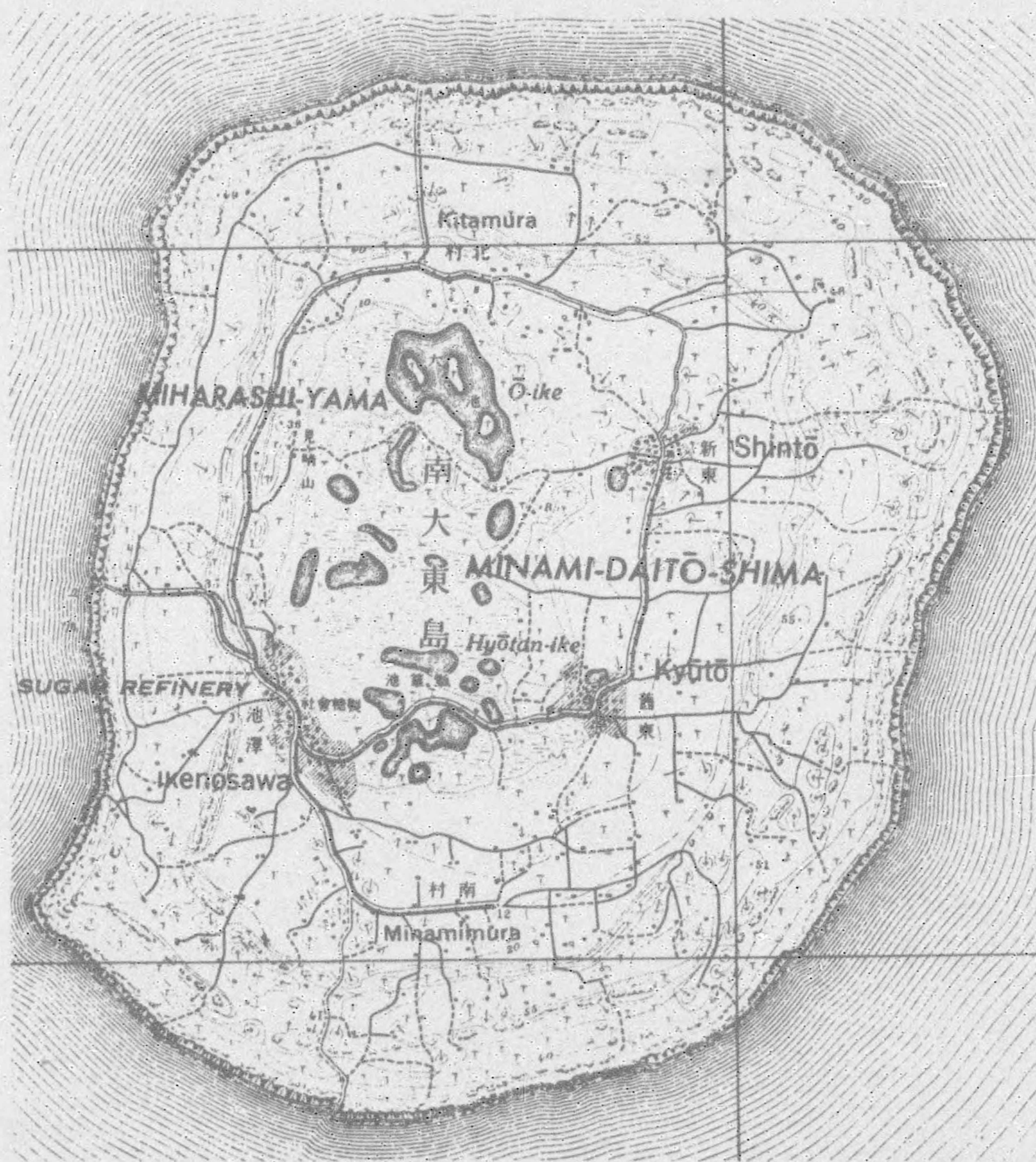
Land in the E. central part of the island, E. of Kyūto, appears suitable for an 8,500-foot field with a N.N.E.-S.S.W. orientation.
