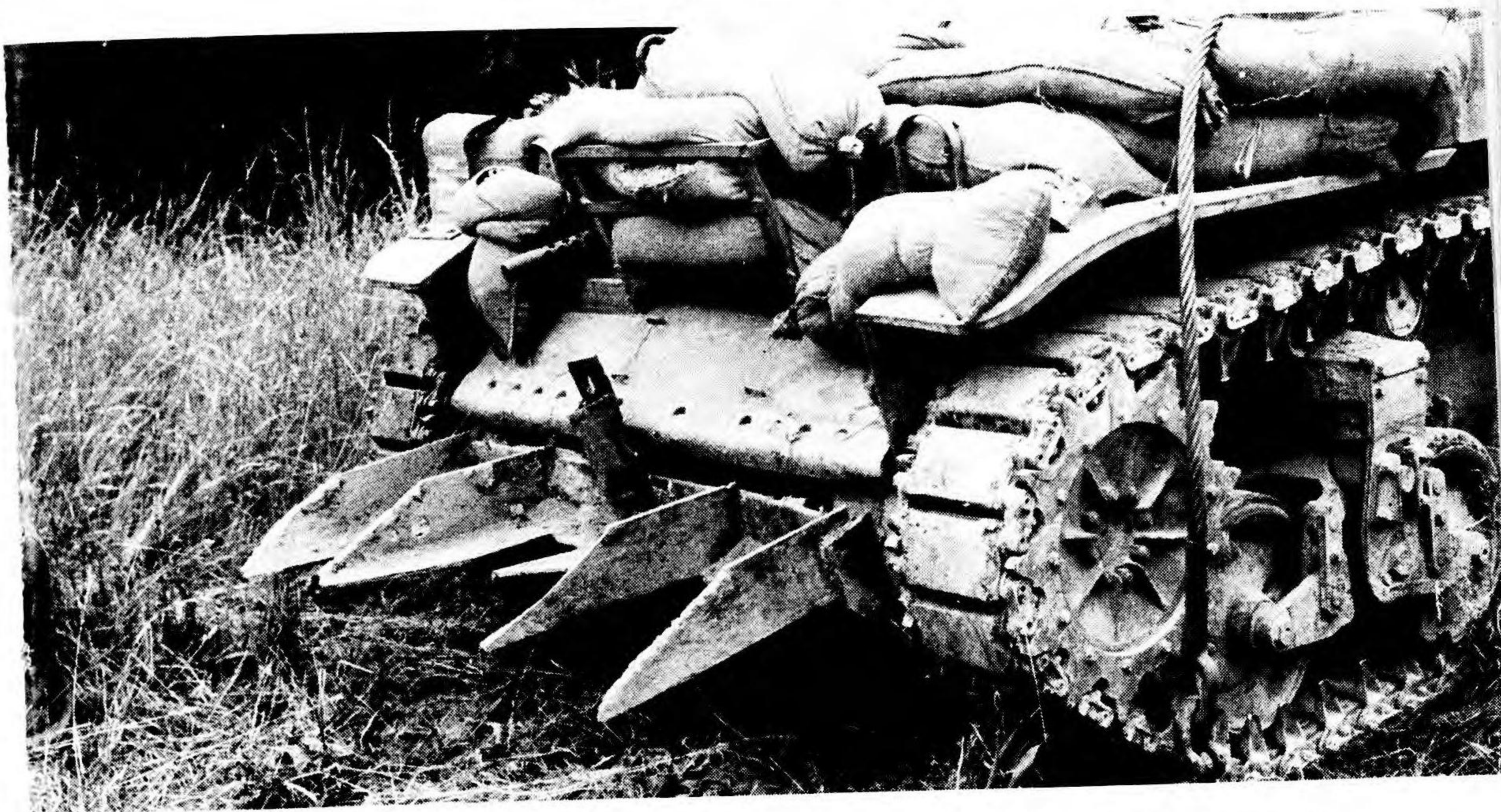
A U. S. light tank fitted out as a hedgerow plow; the cutting edge is provided by metal taken from German beach obstacles. The lower photograph shows a tank going through a hedgerow gap cleared by a bulldozer. (Confidential.)
