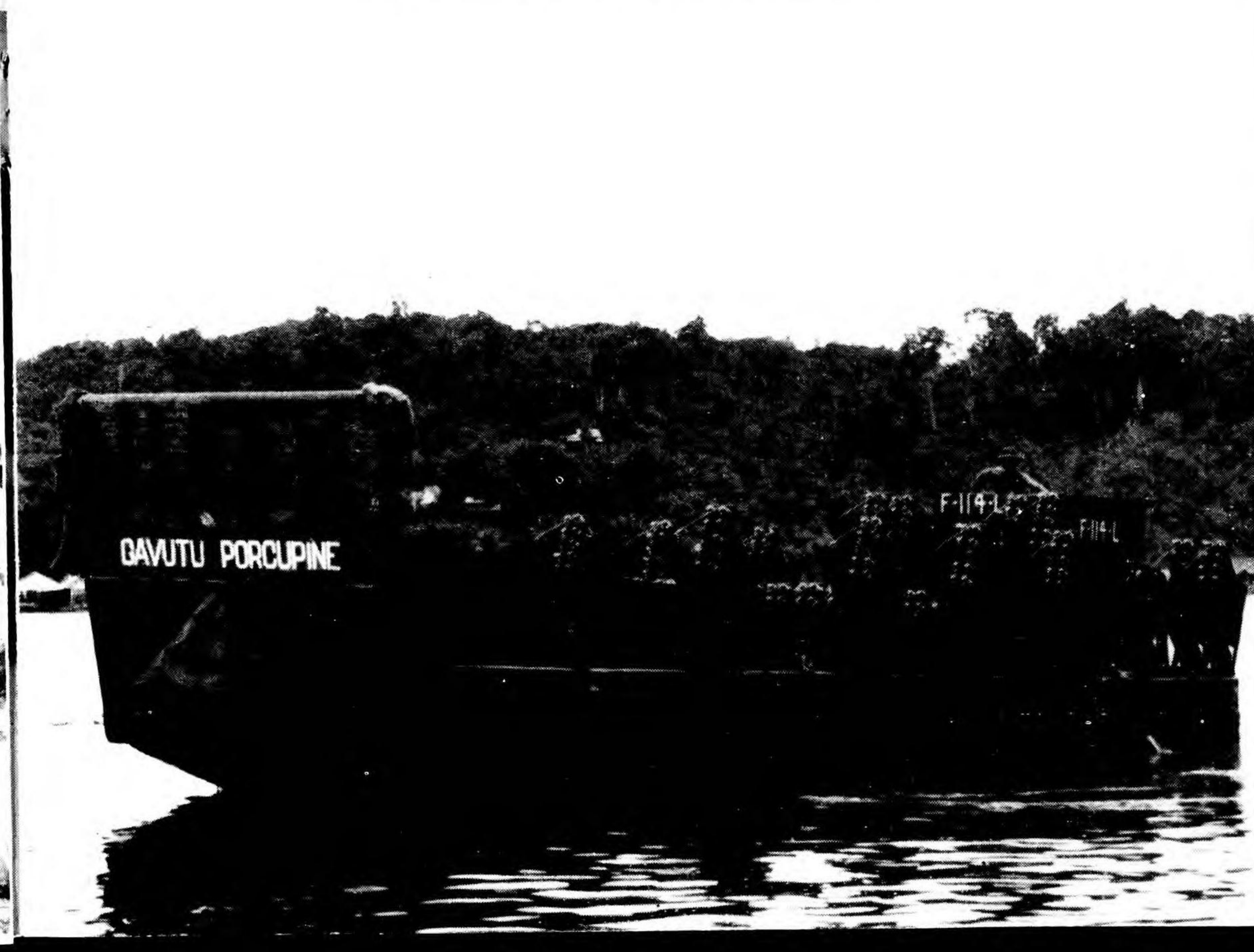
An LCM (3), one of the many types of U. S. landing craft now equipped with rockets; the rocket launchers almost fill the hold. (Confidential!)
