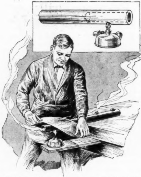
Bending a Strip of Thin Wood over a Polished Axle or Pipe Heated with an Alcohol Lamp
