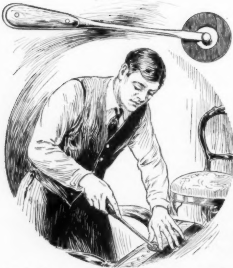
Washer Laid over Tack to Be Pulled Provides Leverage and Prevents Objectionable Marks
