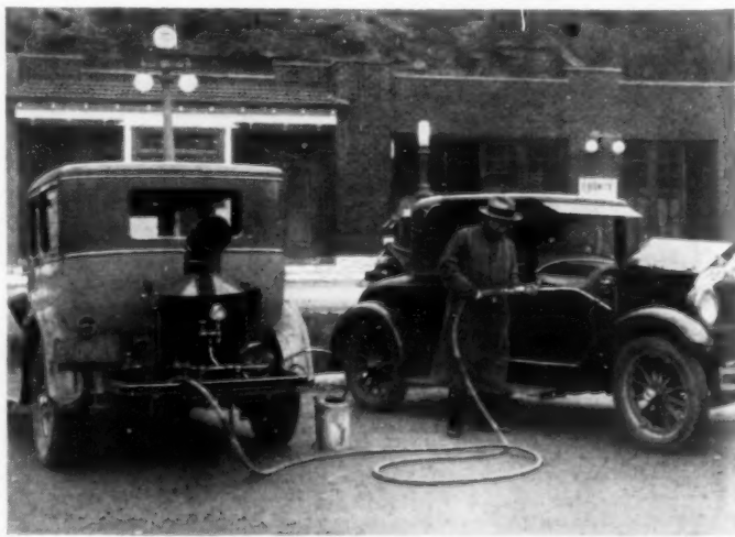
Cleaning Auto Parts with Hot Spray from Generating Unit Attached in Rear of Service Car; High Pressure Is Quickly Developed
