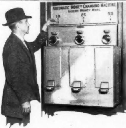
Even Change Can Be Made by Machinery as Well as by a Cashier; the Machine Above Takes Different-Size Coins and Returns Others of the Proper Size to Fit Vending Machines; at the Right, an Automatic Telephone-Call Recorder That Takes Messages While You Are Away
