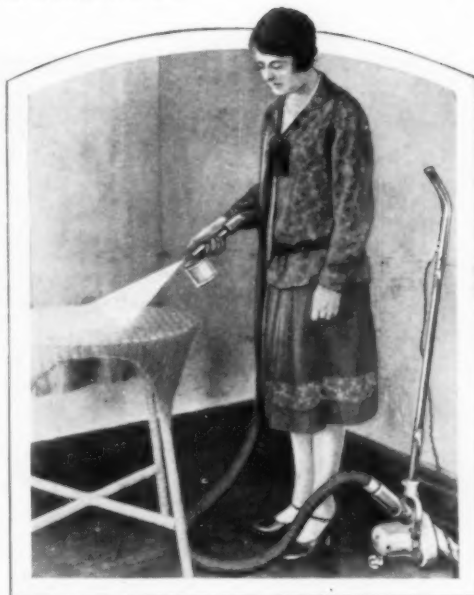
Vacuum Cleaner Rigged as a Sprayer for Furniture or Other Articles
