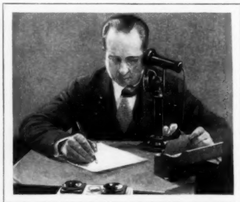
Using the Telephone without the Hands; the Mouthpiece and Receiver Attachment in Service
