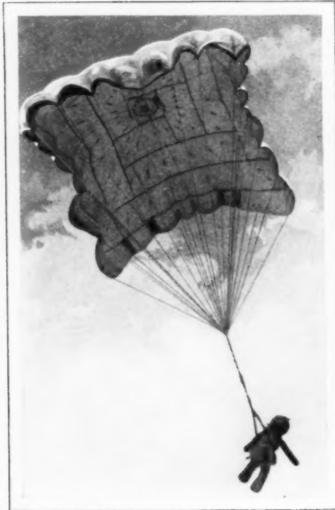
Testing the Square Parachute with Dummy at Lakehurst, N. J.: These Canopies Are Easily Folded
