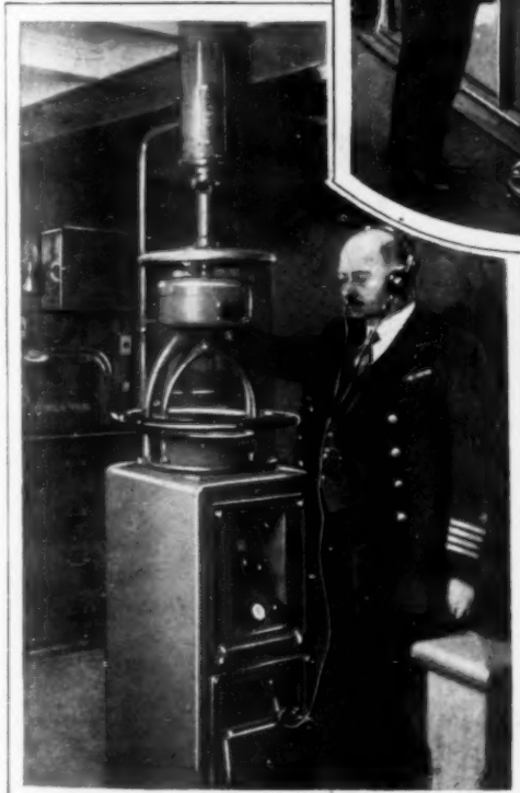
Officer of an Atlantic Liner Listening In As He Turns the Loop of the Radio Direction Finder; Above, the Revolving Sleet-Proof Vision Screen as Used on an Open Bridge
