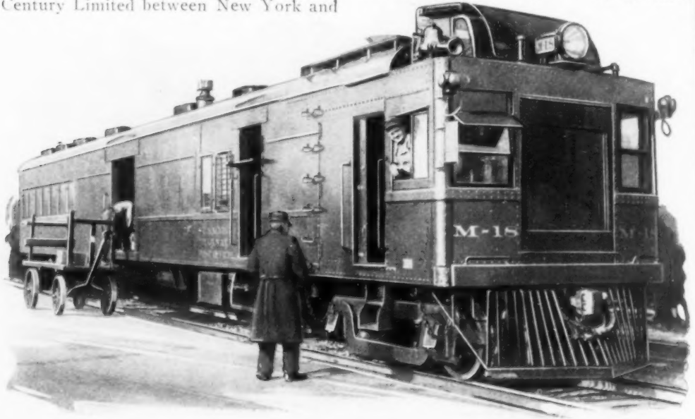
Built to Carry Mail, Express, Baggage and Passengers, and Haul a Trailer or Two if Necessary, the New Gas-Electric Coaches, Capable of Making Sixty-Eight Miles an Hour, Are Displacing Accommodation Trains
