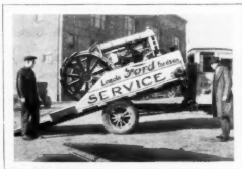
Service Truck with Body Tilted for Handling a Tractor; the Same Arrangement Is Useful in Towing Wrecks
