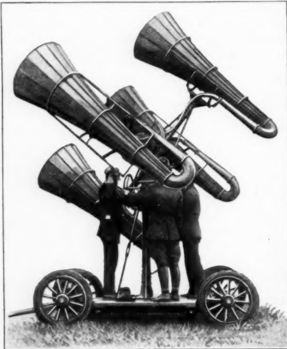
The Ears of the Anti-Aircraft Gunners Are This Battery of Super-Sensitive Sound Collectors
