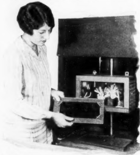
Part of the Ultraviolet-Ray Apparatus in Which Fraudulent Checks and Other Articles Are Detected
