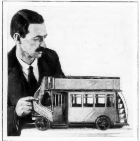
Inventor with Model of the Double-Entrance and Exit Autobus for Rapid Loading and Unloading
