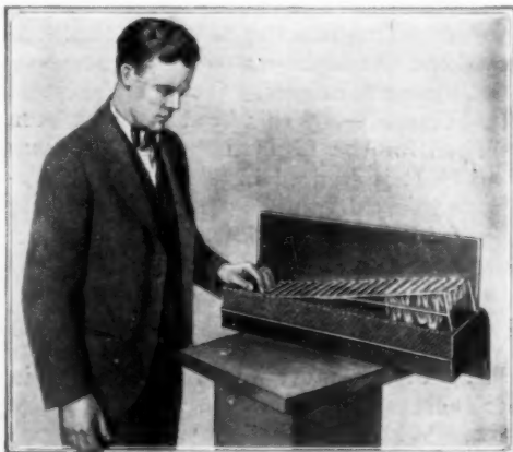
Cloth Wicks in This Radiator Humidifier Absorb Water from Pan and So Increase Evaporation
