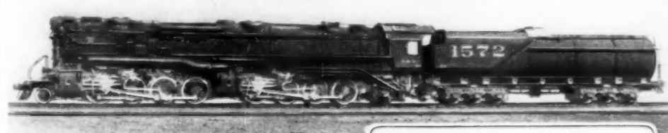
High-Pressure Articulated Locomotive, Above, and, Below, a New British Turbine Engine Which Has Boiler Only in the First Unit and Carries the Driving Mechanism on the Tender; It Is Used in Express Service
