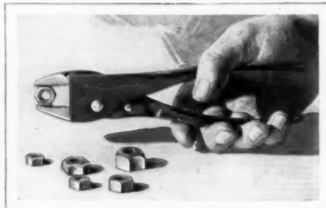
Parallel-Jaw Pliers Employing Double Fulcrum to Increase Gripping Pressure
