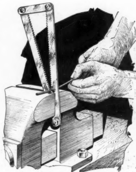
Device Made from Hacksaw Blades Is Useful for Stripping Insulation from Wire
