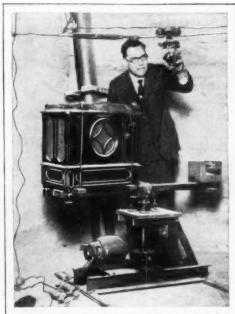
Noise Producer in Use, and Part of the Measuring Apparatus at Bureau of Standards
