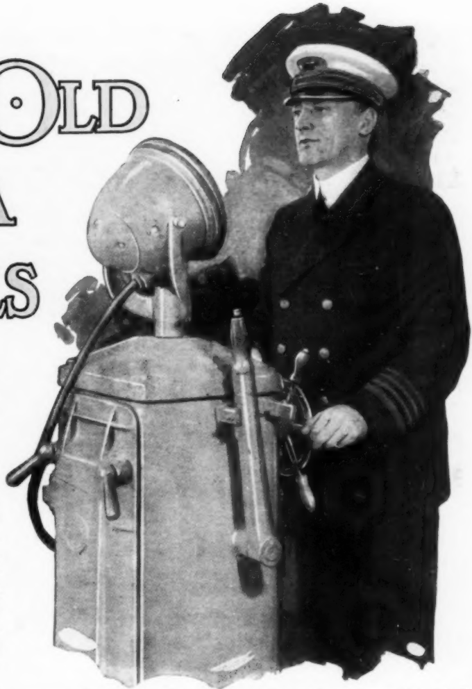
"Metal Mike," Which Guides a Giant Liner without Human Help, Is Set with This Small Wheel
