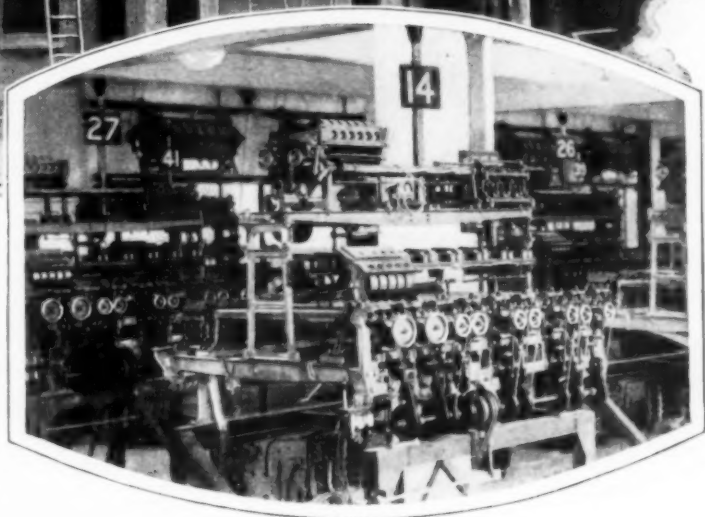
Exterior View of the Betting Announcer, and Glimpse Inside at the Complicated Computing Apparatus Which Quickly Tallies the Odds and Gives the Results
