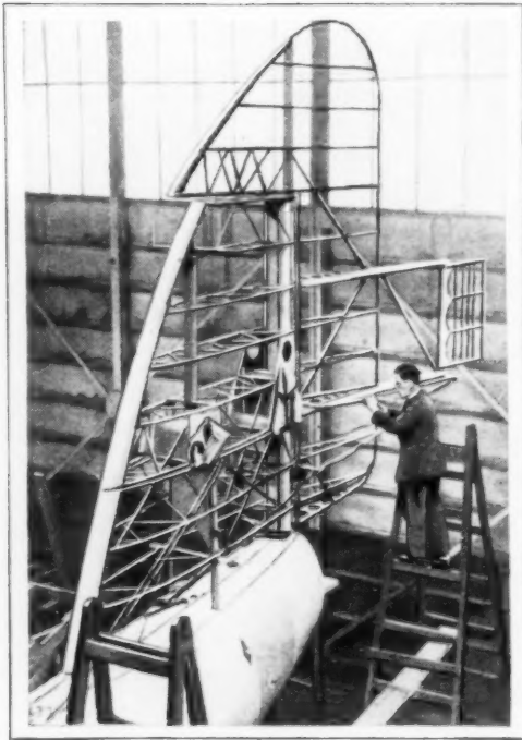
Rudder Skeleton of One of the Huge Air Liners for Service between England and Australia
