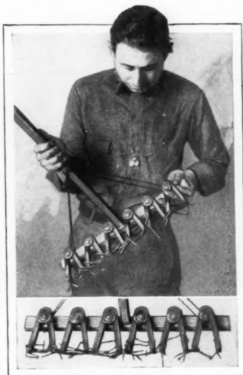
Rake Made from Discarded Magnets Is Useful for Picking Up Nails and Tacks
