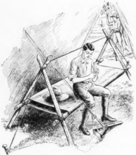
Camper's Bed Consisting of a Doubled Length of Canvas, Which Provides Dead-Air Space
