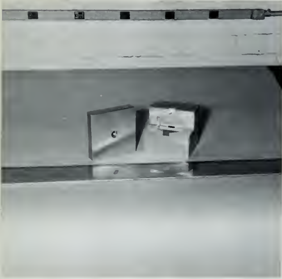
A. Three-piece end block before assembly. Coolant channel in foreground.
