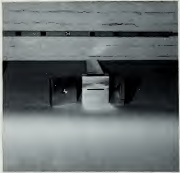
B. Channel end block showing coolant channel slot.
