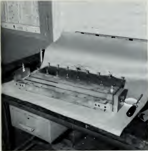
A. Coolant channel inserted into support block.
