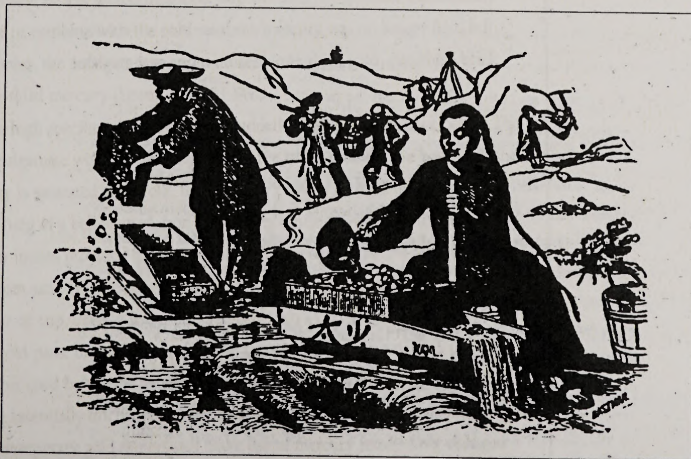
Figure 3.1b. Chinese miners using rocker in California. (Illustration from Hutching's California Magazine, 1856.)
