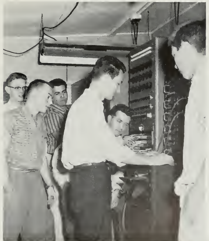
Students take notes from the network analyzer, simulating a system to aid in the solution of difficult problems.
