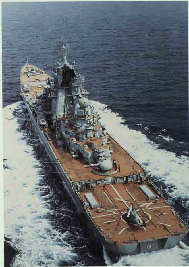
The Soviets have now launched a fourth unit of the 28,000-metric-ton Kirov-class nuclear-powered guided-missile cruiser, which carries 20 SS-N-19 500-km range surface-to-surface missiles as part of its weapons suite.
