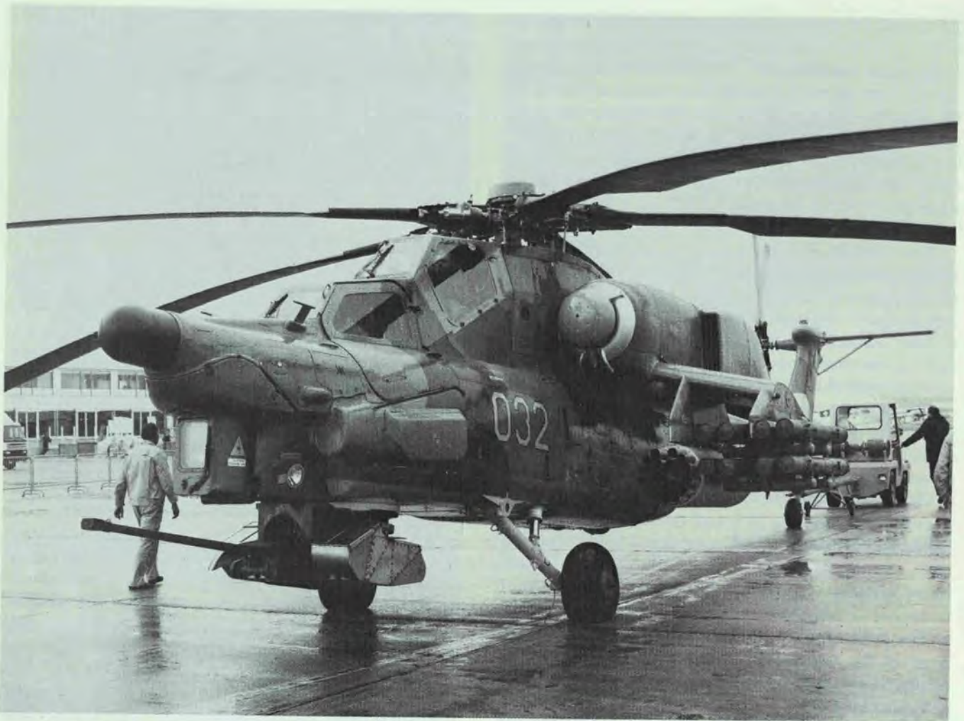
The Mi-28 Havoc, armed with antitank guided missiles, unguided rockets, and a single-barrel gun mounted beneath its forward fuselage, is the USSR's newest attack helicopter.
