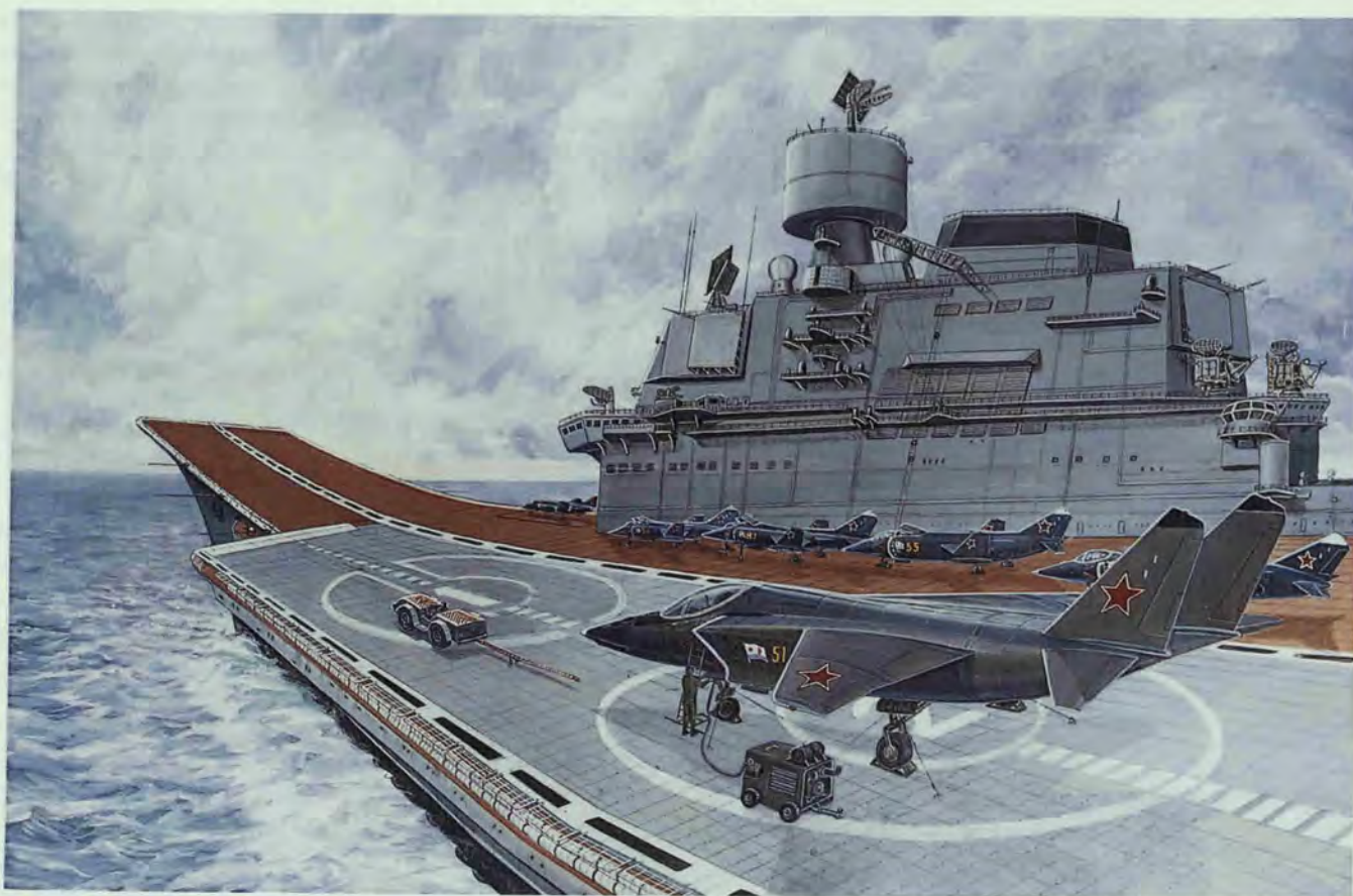
The first unit of the Soviet Union's new 65,000-metric-ton Tbilisi-class aircraft carriers will mark a significant evolutionary advance over the Kiev-class carriers. Candidate aircraft for its intended airwing include the new Yak-41 VSTOL fighter interceptor now in flight test, as well as the Su-27 Flanker. The first Tbilisi-class carrier may begin sea trials this year.
