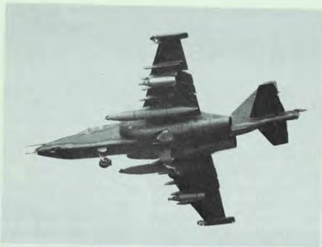
A dedicated ground support fighter, the Su-25/Frogfoot is armed with rockets, antitank missiles, and cannon for its close air support mission.
