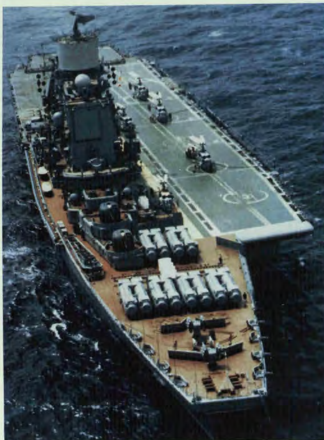
Baku , the fourth unit of the Kiev-class carriers, which carries more sophisticated target acquisition and tracking radars than the other ships of the class, joined the Northern Fleet in 1988.
