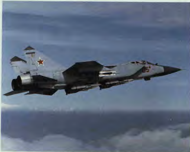
The MiG-31 Foxhound, a fourth-generation Soviet fighter interceptor with a look-down/shoot-down capability, has significantly increased the quality of Soviet air defense forces.
