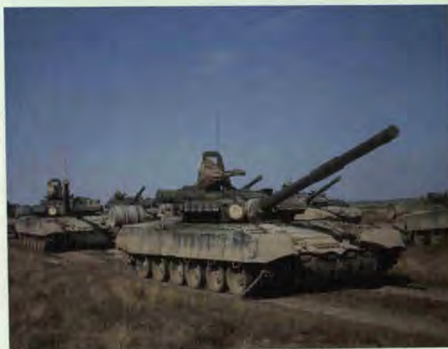
These modern Soviet main battle tanks deployed in Eastern Europe are equipped with reactive armor, which substantially reduces the effectiveness of NATO antitank missiles. Roughly 3,000 modern Soviet tanks are fitted with reactive armor mounting apparatuses.
