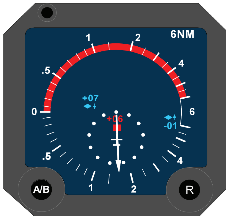
Figure 3C-155. Preventive RA Operational Situation
