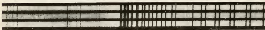
FIG. 3—Lines of B group due to oxygen in the Earth's atmosphere undisplaced by Sun's rotation, red region, \lambda 6867 .
