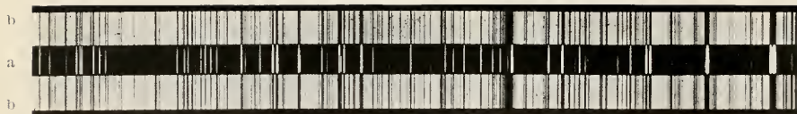
FIG. 1—Coincidence of bright lines (a) from iron vapor with dark lines (b) in the Sun's spectrum, violet region, \lambda 4200 .
