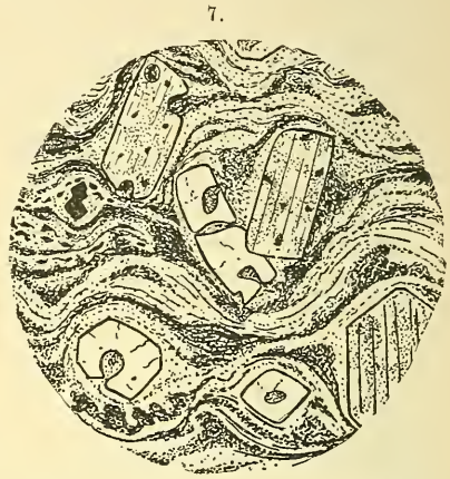
Fig. 7.—Flow structure. No. 61, South of Willow Grove, Pa., mag. 5 diameters.
